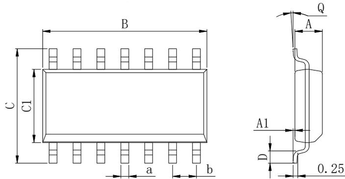
**Dimensions In Millimeters(SOP-14)**
