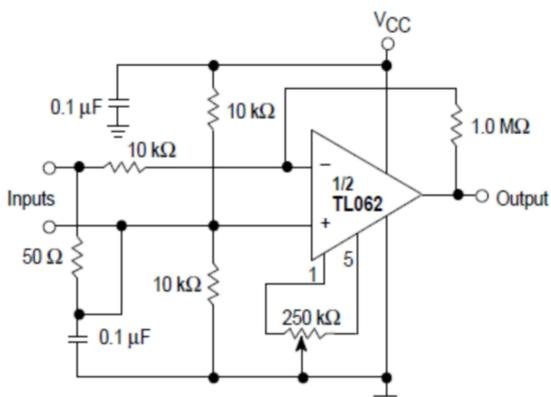
Figure 20. High-Q Notch Filter
