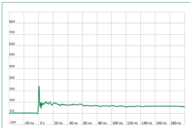
IEC 61000-4-2 +8 kV Contact ESD Clamping Voltage
