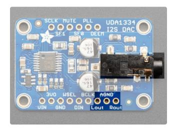
The exciting part! This is where your line level audio comes out. We put big 47uF blocking capacitors on the output so you can connect this to any stereo system.
