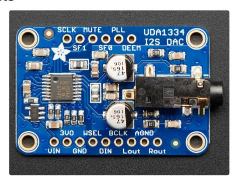
The UDA1334A is an **I2S** amplifier - it does not use analog inputs, it only has digital audio input support! Don't confuse I2S with I2C, I2S is a sound protocol whereas I2C is for small amounts of data.
