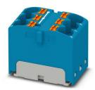
Distribution block, bridged internally, nom. voltage: 450 V, nominal current: 32 A, number of connections: 6, connection method: Push-in connection, cross section: 0.2 mm² - 6 mm², mounting type: for snapping onto a DIN rail adapter, Direct mounting with flange, Free-hanging, color: blue
