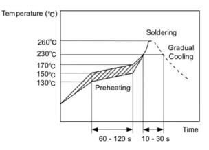
Wave Soldering Curve
