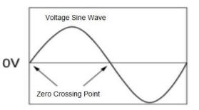
\*Zero crossing refers to the position where the sine wave voltage passes through 0V. See the figure on the right.
