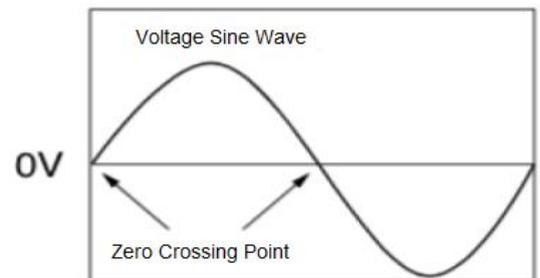
\*Zero crossing refers to the position where the sine wave voltage passes through 0V. See the figure on the right.
