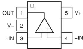
Figure 4-1. OPA328 DBV Package, 5-Pin SOT-23 (Top View)
