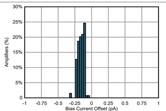
Figure 5-12. Input Bias Offset Current Distribution
