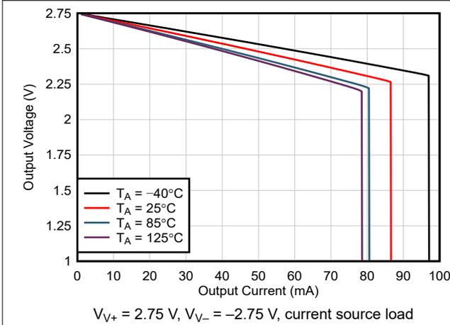
Figure 5-21. Output Voltage Swing vs Output Current
