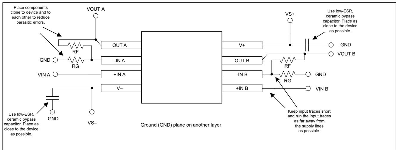
**Figure 7-6. Operational Amplifier Board Layout for Noninverting Configuration**
