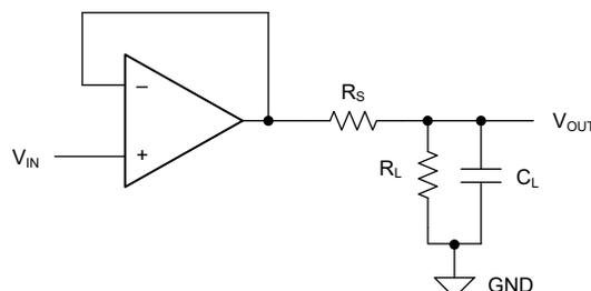
**Figure 7-1. Improving Capacitive Load Drive**
