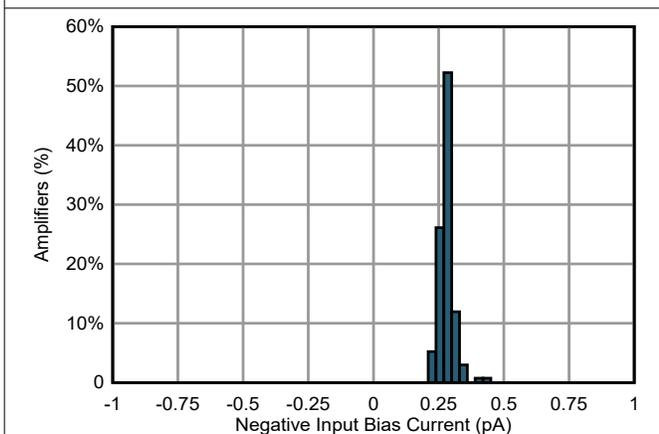
Figure 5-11. Negative Input Bias Current Distribution
