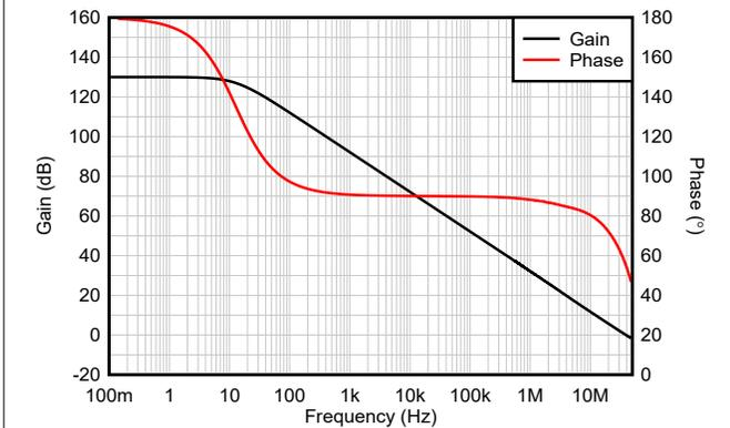
Figure 5-5. Open-Loop Gain and Phase vs Frequency
