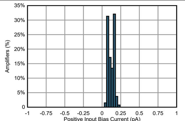
Figure 5-10. Positive Input Bias Current Distribution
