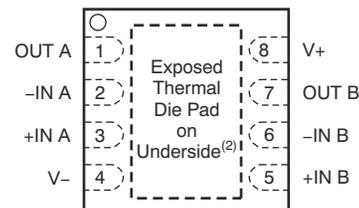
Figure 4-4. OPA2328 DRG Package, 8-Pin WSON (Top View)
