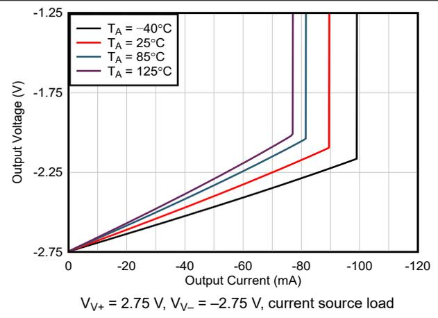
Figure 5-22. Output Voltage Swing vs Output Current
