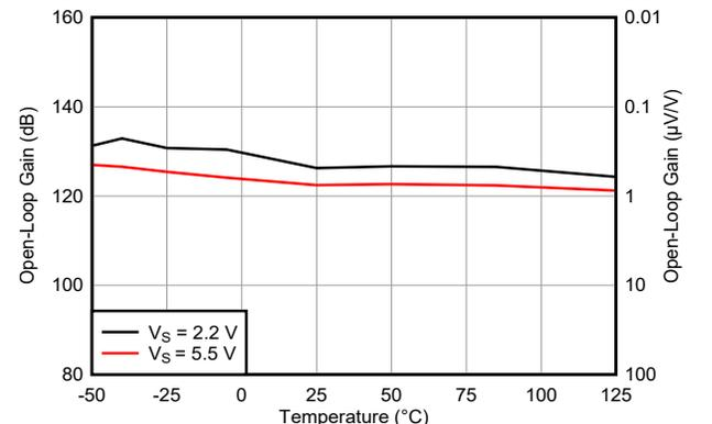
Figure 5-6. Open-Loop Gain vs Temperature
