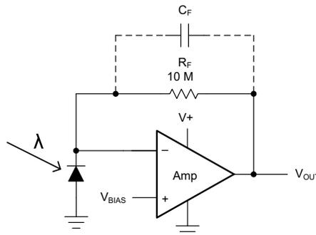
NOTE:  $C_F$  is optional to prevent gain peaking, and includes the stray capacitance of  $R_F$ .
