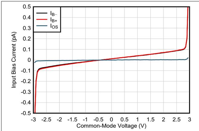
Figure 5-7. Input Bias Current vs Common-Mode Voltage
