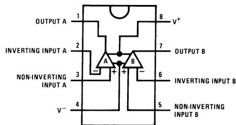
**Figure 2. 8-Pin SOIC (See D Package)
