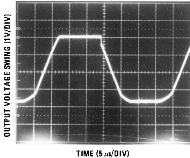
Figure 28. Current Limit ( $R_L = 100\Omega$ )
