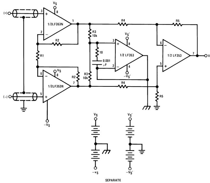
$$A_V = \left( \frac{2R_2}{R_1} + 1 \right) \frac{R_5}{R_4}$$
