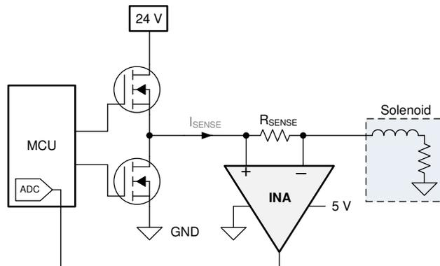
**Figure 30. Current Sensing in a Solenoid Application**
