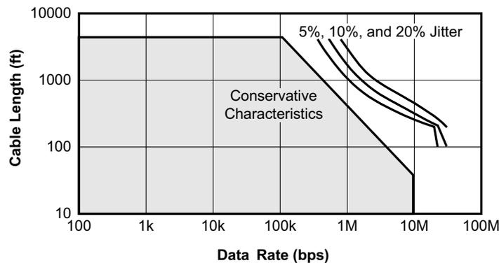
Figure 26. Cable Length vs Data Rate Characteristic
