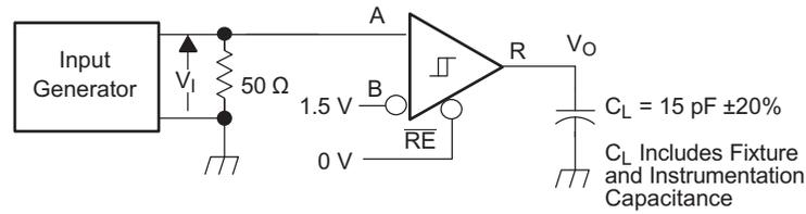
Generator: PRR = 500 kHz, 50% Duty Cycle,  $t_r < 6 \text{ ns}$ ,  $t_f < 6 \text{ ns}$ ,  $Z_o = 50 \Omega$
