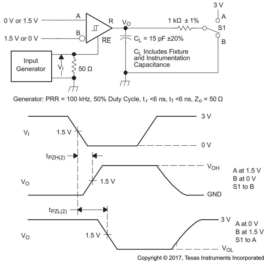
Figure 21. Receiver Enable Time From Standby (Driver Disabled)
