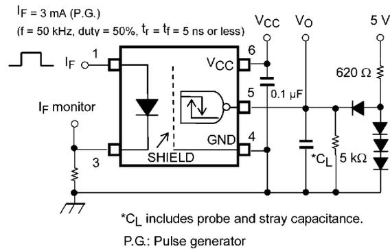
**Fig. 12.1.7 Switching Time Test Circuit and waveform**
