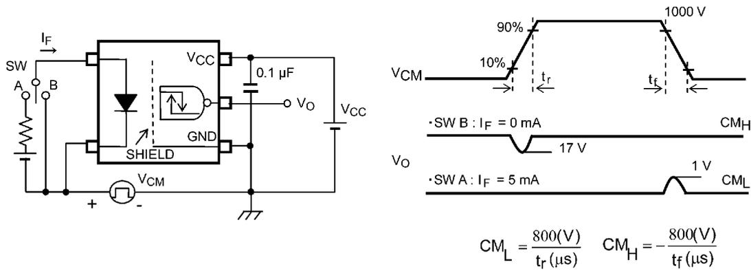
Fig. 12.1.9 Common-Mode Transient Immunity Test Circuit and waveform
