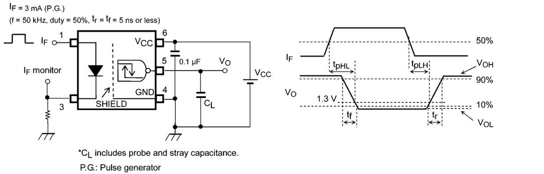
Fig. 12.1.8 Switching Time Test Circuit and waveform
