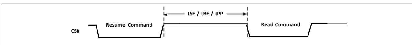
Figure-38. Program Resume and Erase Resume Sequence Diagram
