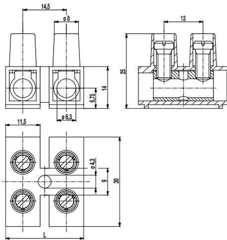
The socket terminal strip 327 is available in 14,5 mm pitch with 1- to 12-pole design and can be easily stripped to the desired number of poles. Due to the M5 screw, the socket hole diameter of 6,3 mm and a creepage distance of more than 9 mm between terminal body and mounting surface, this version is well suited for large cross-sections, high currents and voltages.
