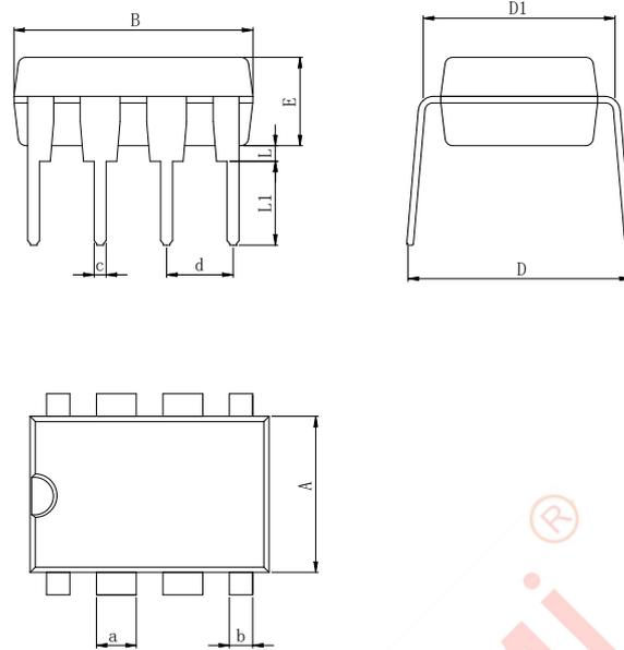
**Dimensions In Millimeters(DIP8L)**
