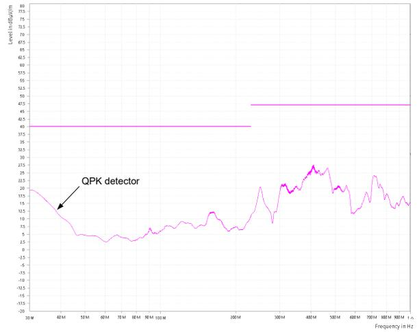
**图 9-9. CISPR 32 Class B Radiated Emissions:
