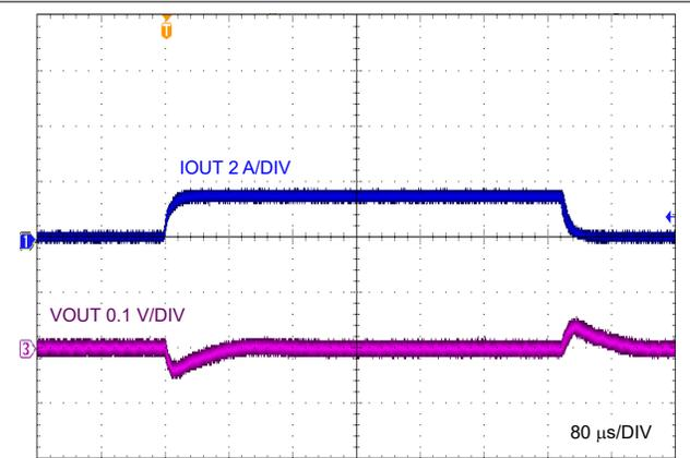
图 9-14. Load Transient, 0 A to 1.5 A
