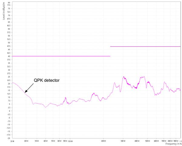
**图 9-8. CISPR 32 Class B Radiated Emissions:
