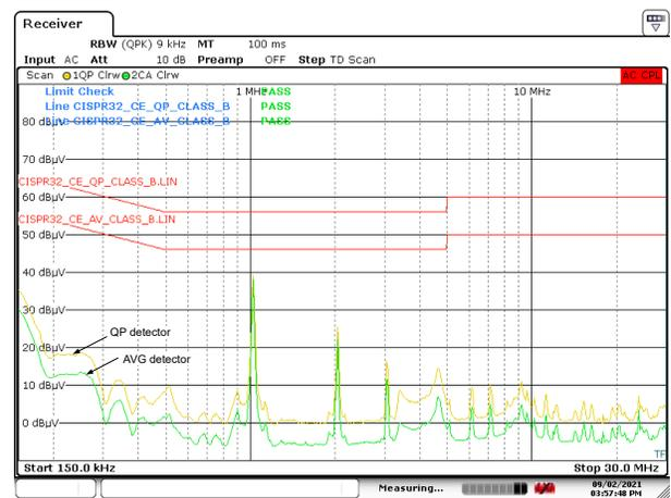
图 9-7. CISPR 32 Class B Conducted Emissions:
