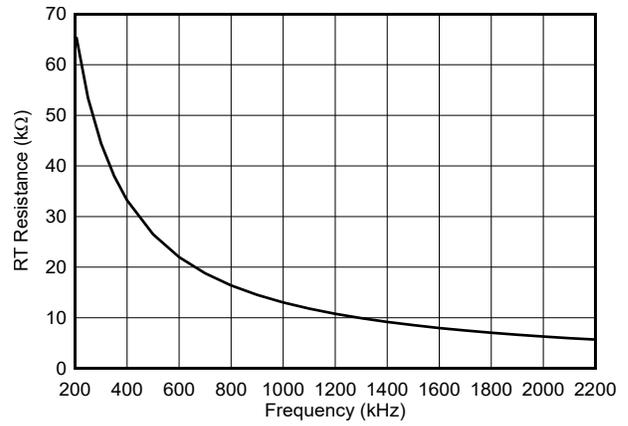
图 7-8. Switching Frequency Set by RT Resistor
