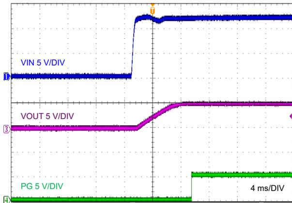
图 9-4. Start-Up,  $V_{IN}$  Stepped to 12 V
