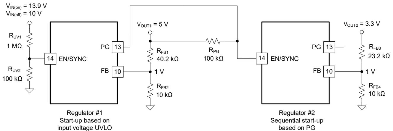
图 8-3. TPSM63604 Sequencing Implementation Using PG and EN/SYNC
