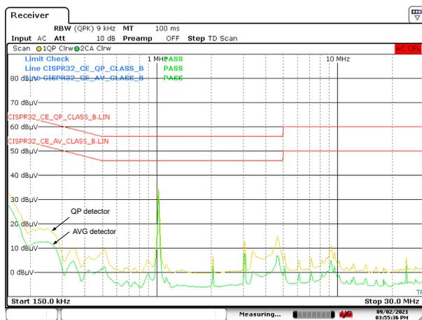
图 9-6. CISPR 32 Class B Conducted Emissions:
