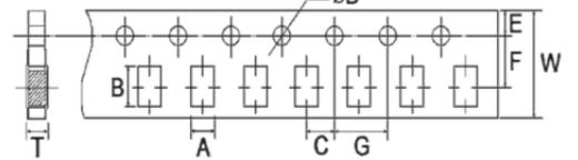
13.2 Dimension of plastic taping: (Unit: mm)
