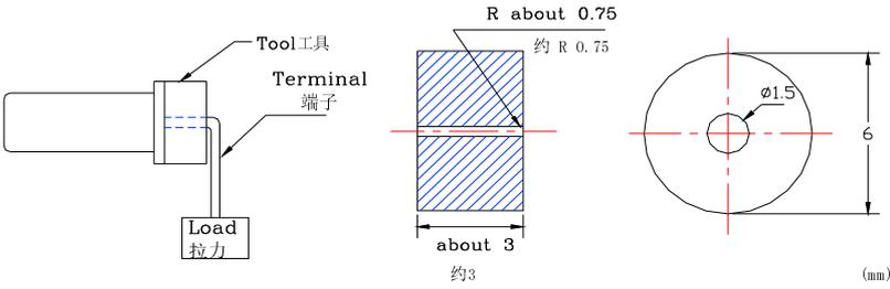
The diagram shows a side view of a specimen being pulled by a tool, a top view of a rectangular specimen with a central hole, and a circular cross-section of the hole. Labels include 'Tool 工具', 'Terminal 端子', 'Load 拉力', 'R about 0.75', '约 R 0.75', 'about 3', '约3', 'ø1.5', '6', and '(mm)'.<br>FIG-1 |
