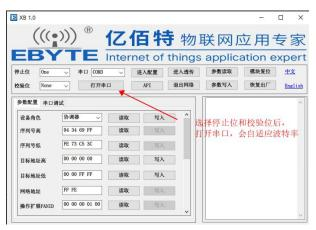
2. After opening the serial port successfully, click to enter the configuration and click API.
