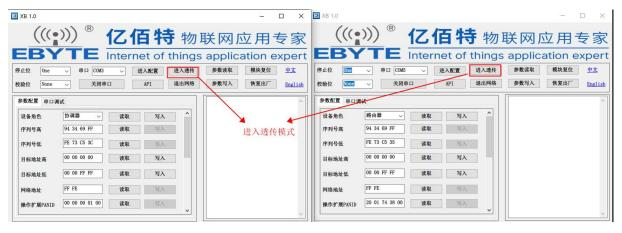
Click serial debugging, in the serial debugging interface, select the frame type as transparent transmission, then enter hexadecimal data in the sending box, and click send to realize transparent transmission communication.
