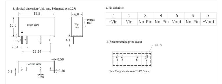
\*Note: If the definition of each pin of the power module is inconsistent with the selection manual, the label on the physical label shall prevail.
