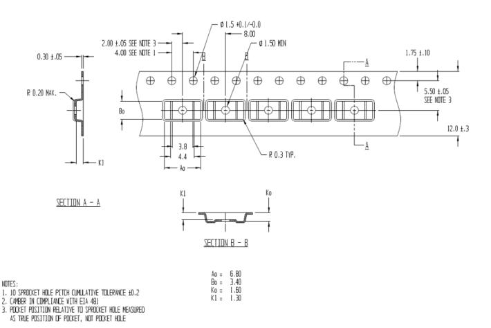
Figure 20: TSSOP-8 Tape and Pocket Drawings
