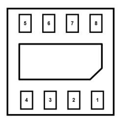
Figure 4: DFN-8, Bottom-Up View
