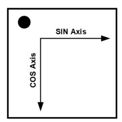
Figure 5: CT310 Axes of Sensitivity for DFN-8
