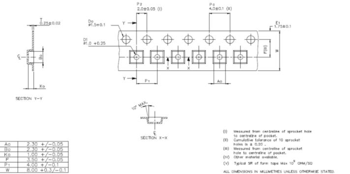
Figure 21: DFN-8 Tape and Pocket Drawings
