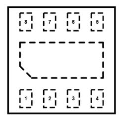
Figure 3: DFN-8,Top-Down View
