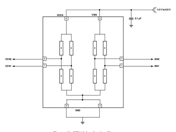
Figure 13: CT310 Application Diagram
