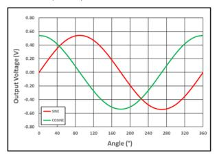
Figure 8: Output Voltage vs. Angle at B = 900 G
