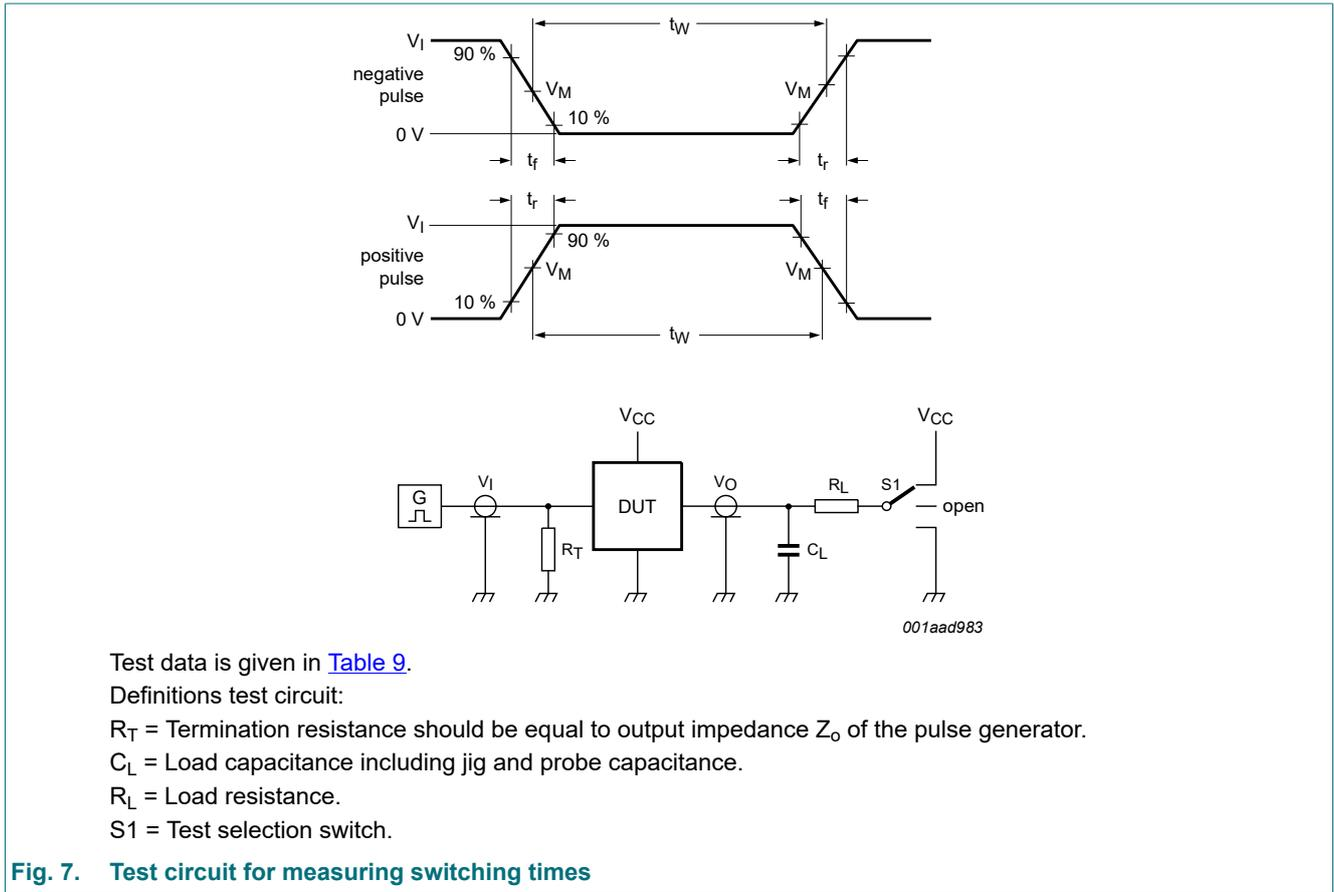
Fig. 7. Test circuit for measuring switching times
