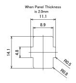
A chamfer of C0.1 is required in order to prevent scrappage to the cover case during panel installation. Number of panel installation can be used up to 10 times.
