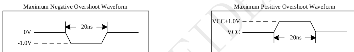
Figure 5-2 Input Test Waveforms and Measurement Level
