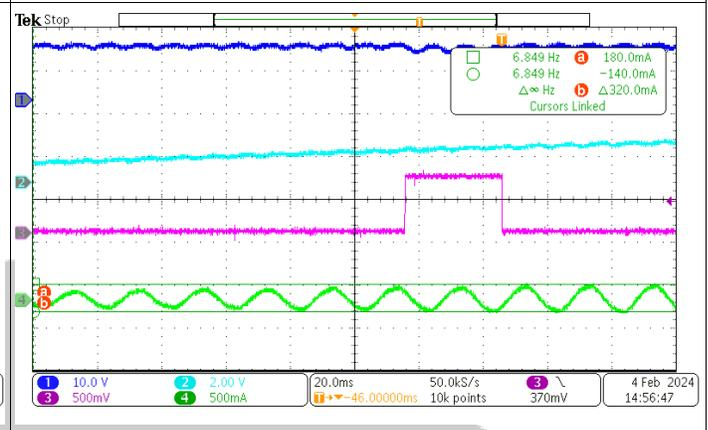
CH1: VS(PIN8),10V/div CH2: OA(Pin5),2V/div
