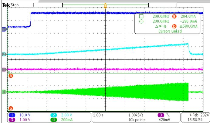
CH1: VS(PIN8), 10V/div CH2: OA(Pin5),2V/div
