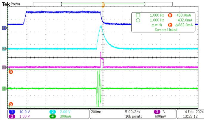
CH1: VS(PIN8),10V/div CH2: OA(Pin5),2V/div
