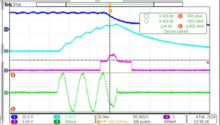
CH1: VS(PIN8),10V/div CH2: OA(Pin5),2V/div
