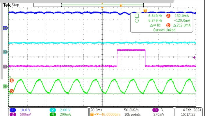
CH1: VS(PIN8),10V/div CH2: OA(Pin5),2V/div
