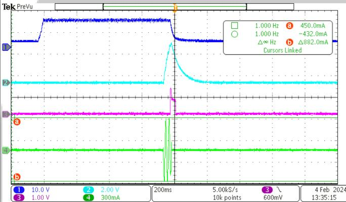
CH1: VS(PIN8),10V/div CH2: OA(Pin5),1V/div
