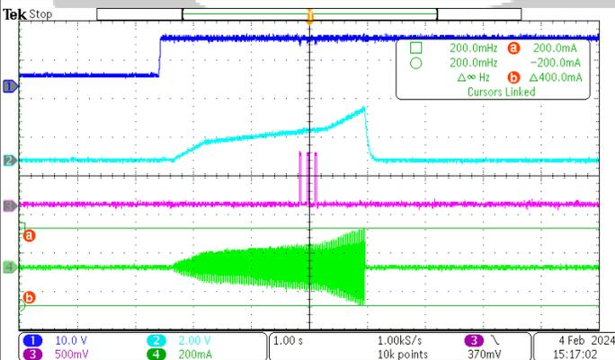
CH1: VS(PIN8),10V/div CH2: OA(Pin5),2V/div
