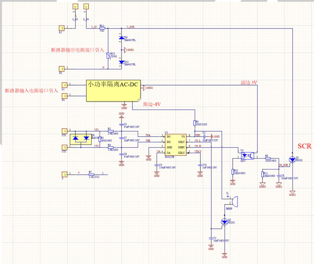
Figure 9. SS4125B high performance application with Beep Warning
