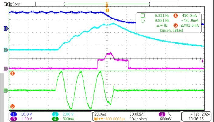
CH1: VS(PIN8),10V/div CH2: OA(Pin5),1V/div
