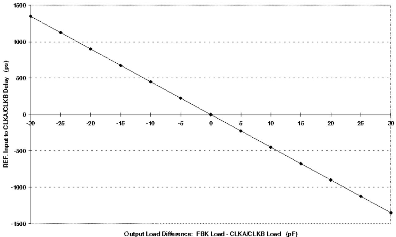
To close the feedback loop of the CY2308, the user has to connect any one of the eight available output pins to FBK pin. The output driving the FBK pin drives a total load of 7 pF plus any additional load that it drives. The relative loading of this output to the remaining outputs adjusts the input-output delay as shown in the [Figure 2](#).
