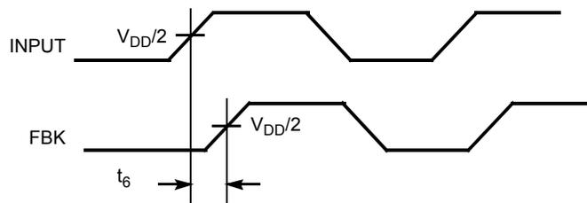
**Figure 7. Device-Device Skew**
