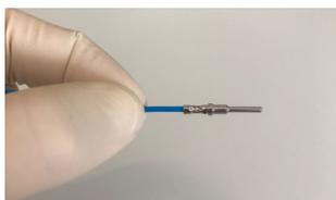
Use a previously crimped contact and wire and hold just behind the contact barrel.
