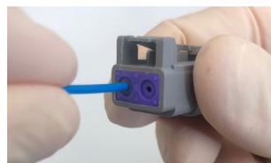
Push the contact until a click is felt. Check the contact is in place by gently tugging and confirming alignment. Repeat for number of contacts desired
