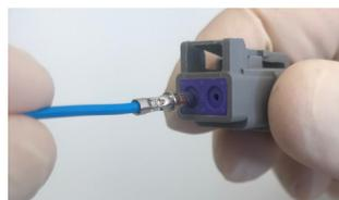
Line the contact up with the grommet.
