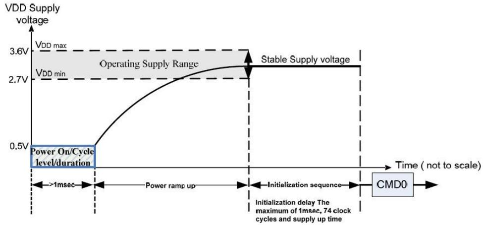
Host needs to keep power line level less than 0.5V and more than 1ms before power ramp up.
