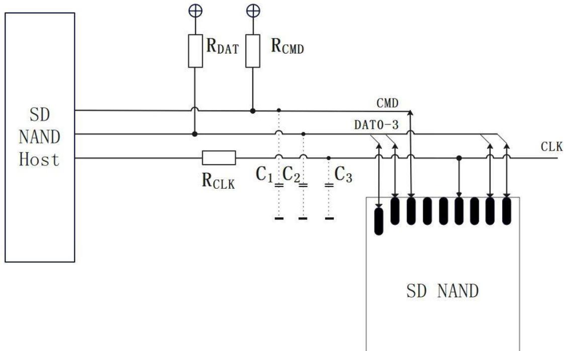
$R_{DAT}$  and  $R_{CMD}$  (10K~100 k $\Omega$ ) are pull-up resistors protecting the CMD and the DAT lines against bus floating when SD NAND is in a high-impedance mode.
