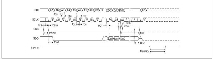
Figure 11. Detailed SPI Timing Diagram
