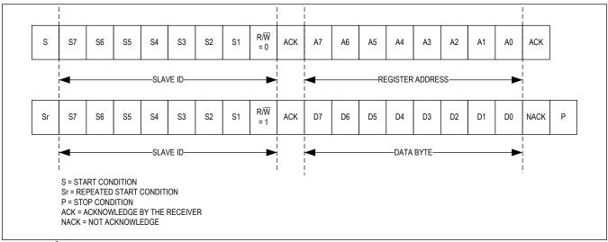
Figure 20. I<sup>2</sup>C Single Byte Read Transaction
