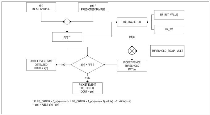
Figure 9. Picket Fence Function Flow
