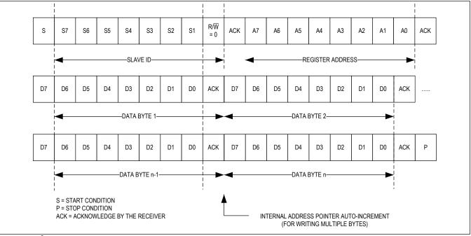
Figure 19. I<sup>2</sup>C Multi-Byte Write Transaction
