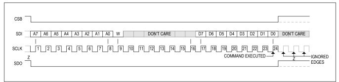
Figure 12. SPI Write Transaction
