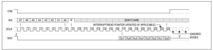
Figure 13. SPI Read Transaction
