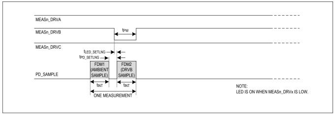
Figure 3. Measurement with FDM
