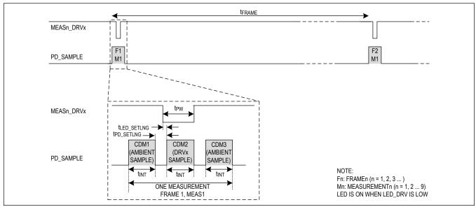
Figure 4. Frame with One Measurement
