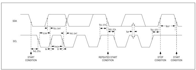
Figure 15. Detailed I<sup>2</sup>C Timing Diagram
