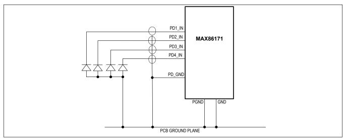
Figure 22. PCB Layout Recommendation
