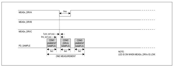
Figure 2. Measurement with CDM
