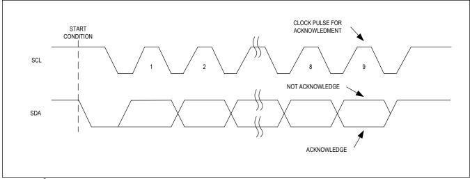
Figure 17. I<sup>2</sup>C Acknowledge Bit
