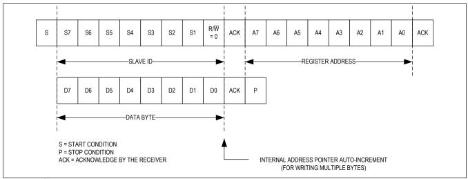
Figure 18. I<sup>2</sup>C Single Byte Write Transaction
