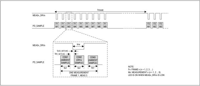
Figure 5. Frame with Nine Measurements
