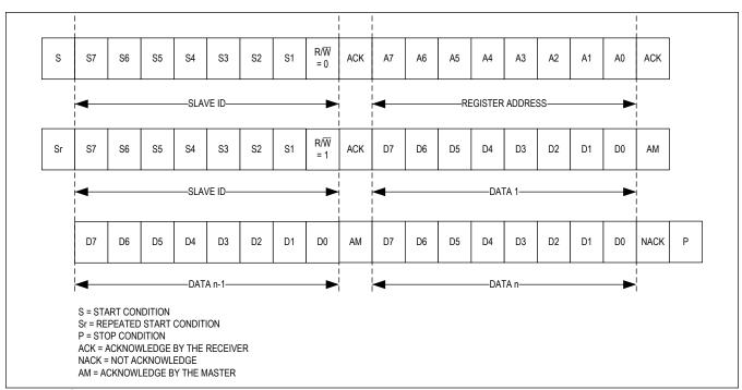
Figure 21. I<sup>2</sup>C Multi-Byte Read Transaction
