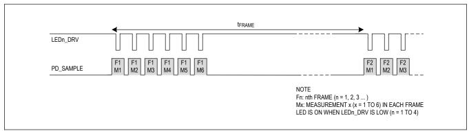
Figure 7. Frame with Six Measurements
