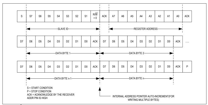
Figure 21. I<sup>2</sup>C Multi-Byte Write Transaction
