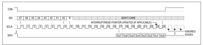
Figure 15. SPI Read Transaction
