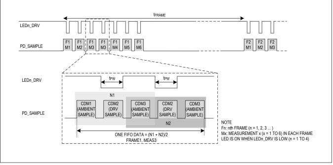
Figure 9. Illustration of Measurement with Burst Averaging
