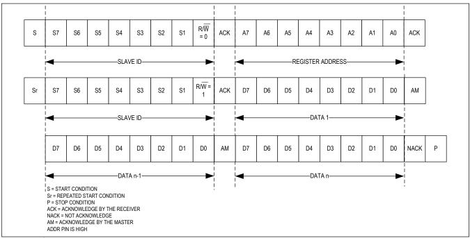
Figure 23. I<sup>2</sup>C Multi-Byte Read Transaction
