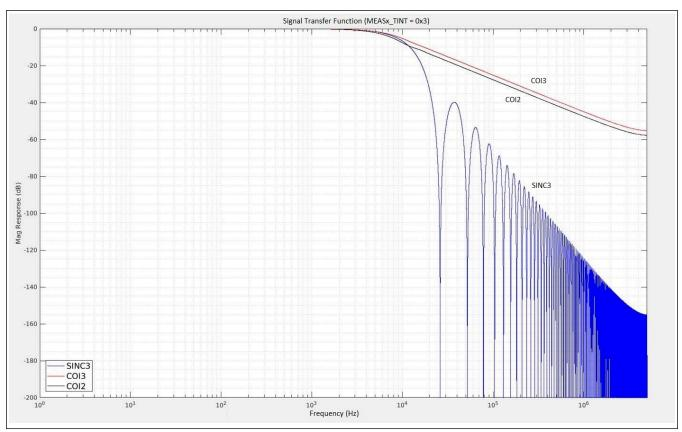
Figure 11. Signal Transfer Function of Decimation Filters
