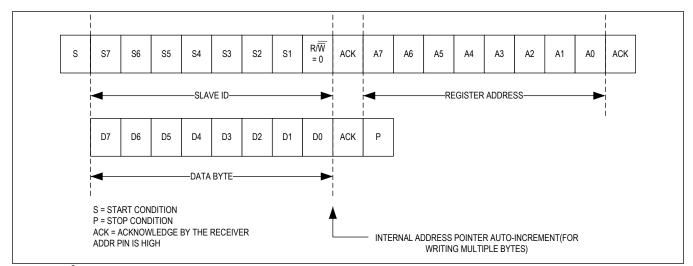
Figure 20. I<sup>2</sup>C Single Byte Write Transaction
