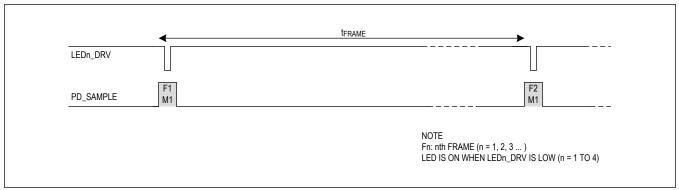
Figure 6. Frame with One Measurement
