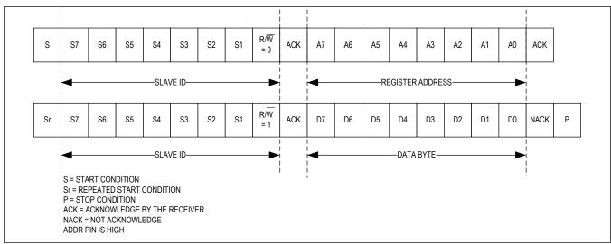
Figure 22. I<sup>2</sup>C Single Byte Read Transaction
