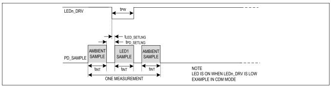
Figure 3. Measurement with One LED On
