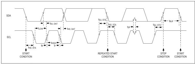
Figure 17. Detailed I<sup>2</sup>C Timing Diagram
