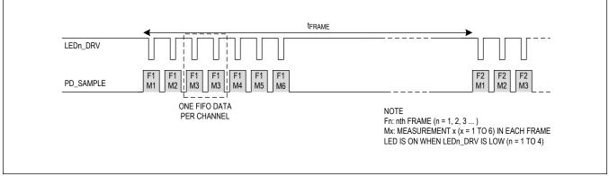
Figure 8. Frame with Measurement Burst Averaging
