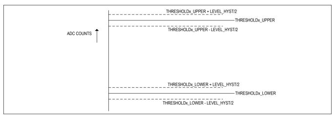
Figure 12. Threshold limits with LEVEL\_HYST
