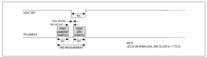
Figure 5. Forward Difference Method (FDM)
