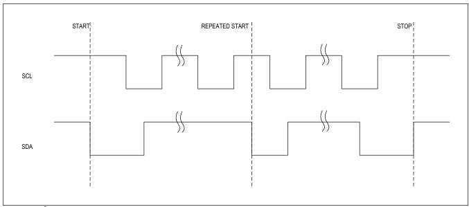
Figure 18. I<sup>2</sup>C START, STOP, and REPEATED START Conditions
