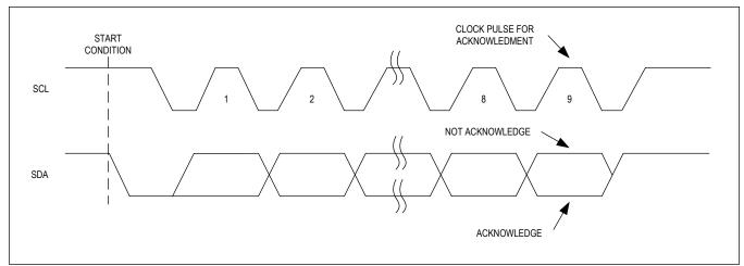
Figure 19. I<sup>2</sup>C Acknowledge Bit
