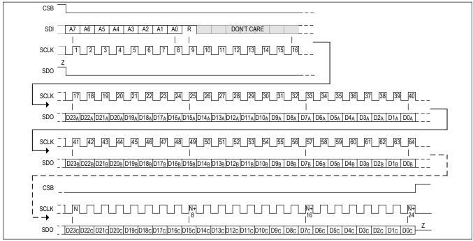
Figure 16. SPI FIFO Burst Mode Read Transaction
