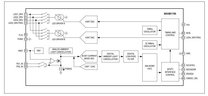
Best-in-Class Optical Pulse Oximeter and Heart-Rate Sensor AFE for Wearable Health
