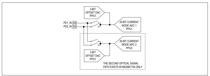
Figure 2. On-Chip Mux for the PD1\_IN and PD2\_IN pins
