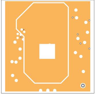
Figure 25. Layer 5—Pseudo PD\_GND Shields PD\_IN
