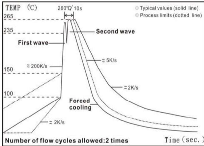
■ **Solder reflow Temperature condition**
