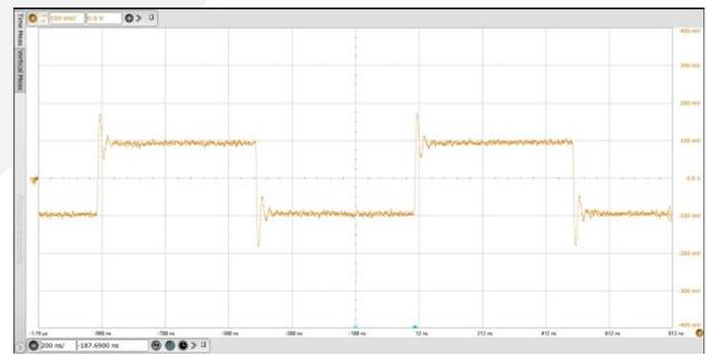
**Figure 10. Small signal step response**
