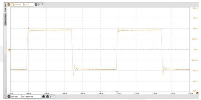
**Figure 12. Large signal step response**
