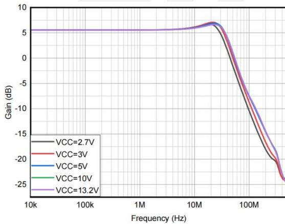
Figure 5. Closed loop frequency response for various supplies
