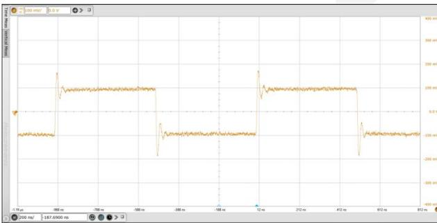
**Figure 9. Small signal step response**
