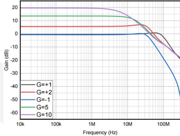
Figure 2. Closed loop gain vs. frequency for various gain
