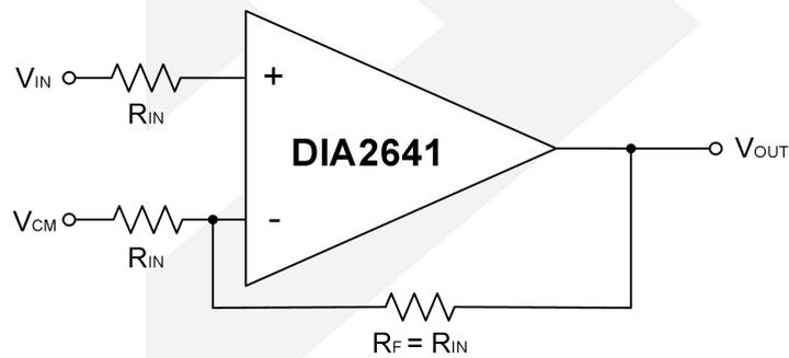
Figure 14. Typical application: gain = 2
