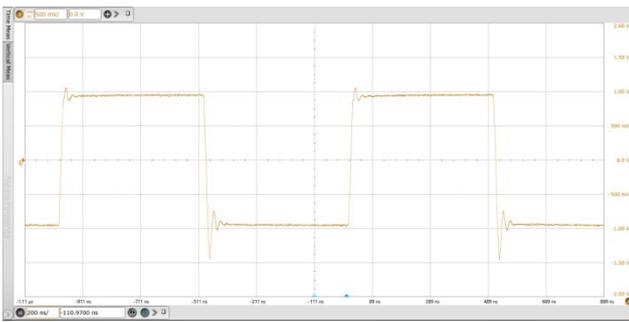
**Figure 11. Large signal step response**
