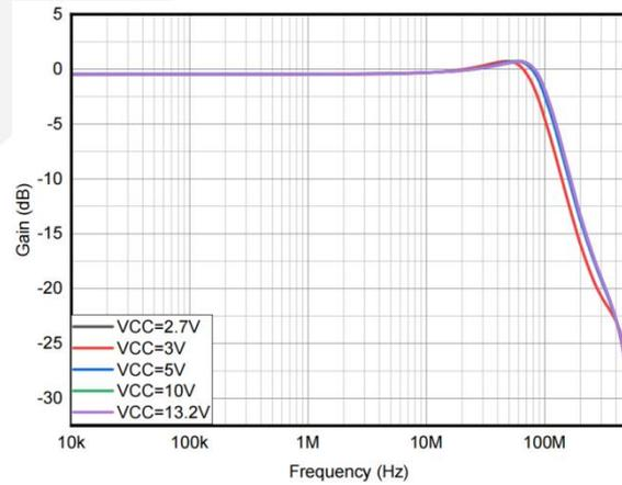
Figure 4. Closed loop frequency response for various supplies
