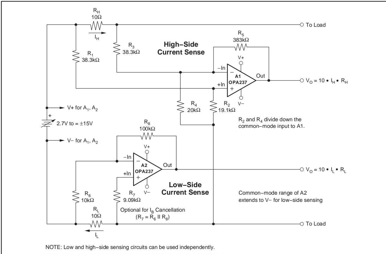
Figure 2. Low and High-Side Battery Current Sensing
