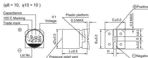
※1. Voltage mark for 6.3V is 「6V」. In case of marking for φ3 units, 「V」 for rated voltage is omitted.
