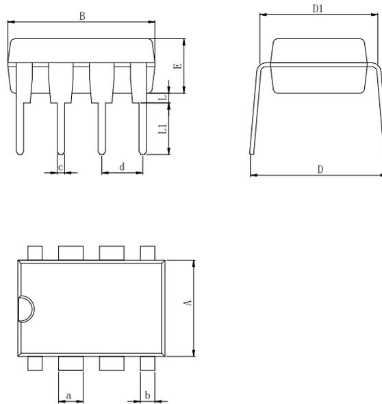
**Dimensions In Millimeters(DIP-8)**
