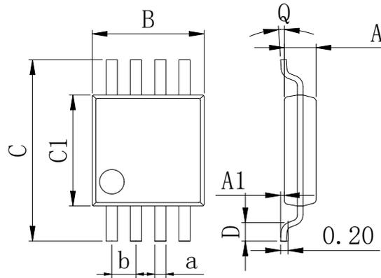
**Dimensions In Millimeters(MSOP-8)**
