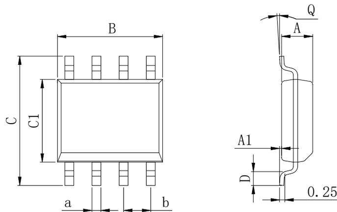
**Dimensions In Millimeters(SOP-8)**
