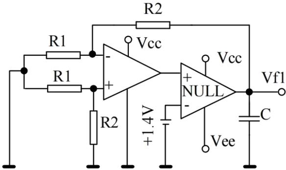
$V_{io} = V_{f1} / (1 + R_2/R_1)$
