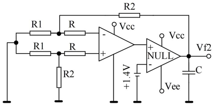
$I_{io} = (V_{f2} - V_{f1}) / R (1 + R_2/R_1)$
