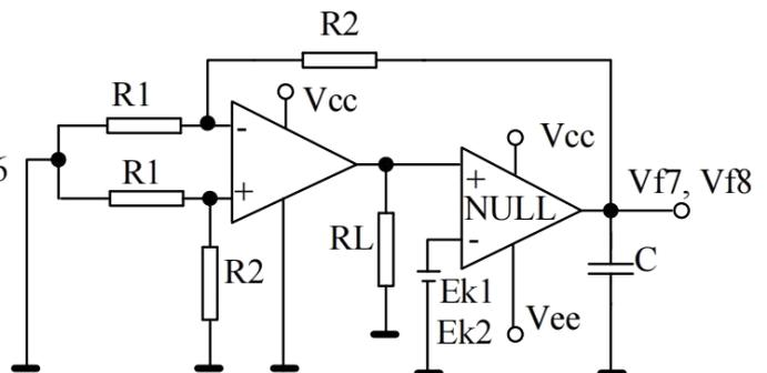
$G_v = (E_{k1} - E_{k2}) (1 + R_2/R_1) / (V_{f7} - V_{f8})$
