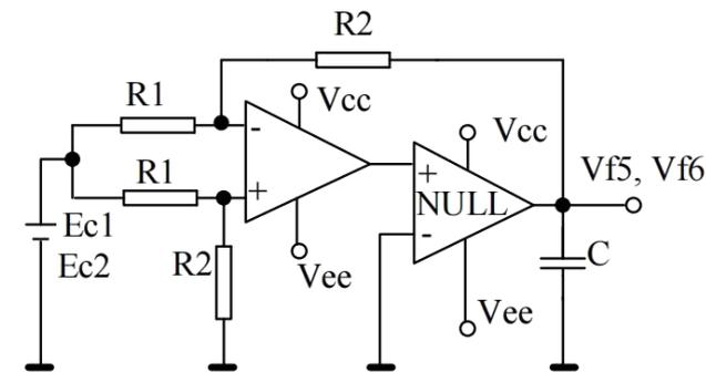
$CMR = 20 \log \left| \frac{(E_{c1} - E_{c2}) (1 + R_2/R_1)}{(V_{f5} - V_{f6})} \right|$
