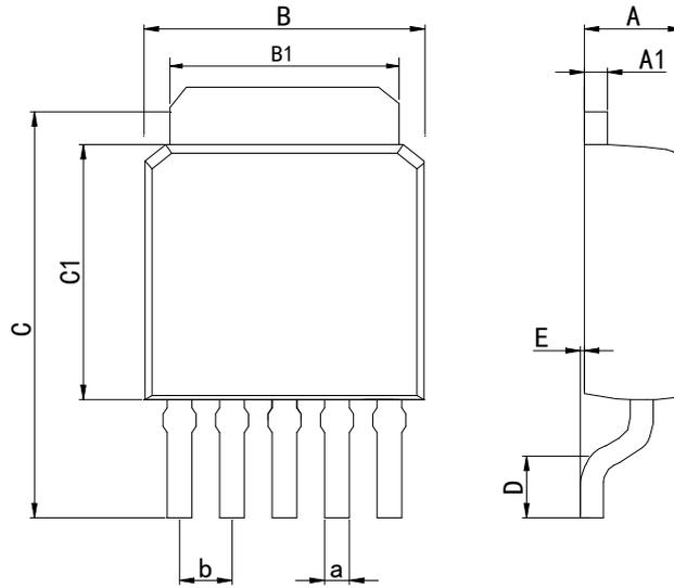
Dimensions In Millimeters(TO-252-5)
