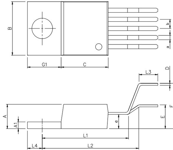
Dimensions In Millimeters(TO220B-5)
