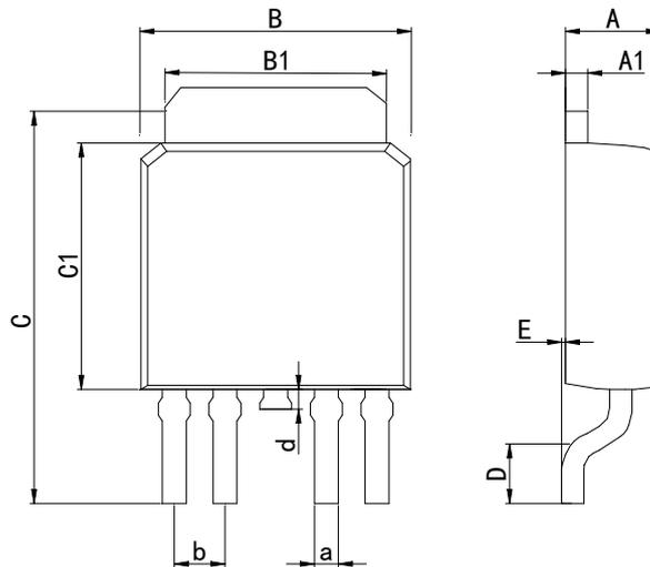
Dimensions In Millimeters(TO-252-4)
