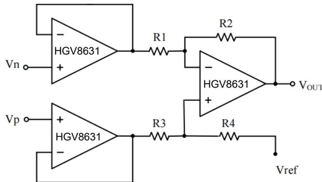
Figure 5. Instrumentation Amplifier
