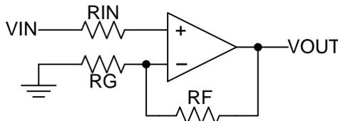
Figure 7. Operational Amplifier Schematic for Noninverting Configuration
