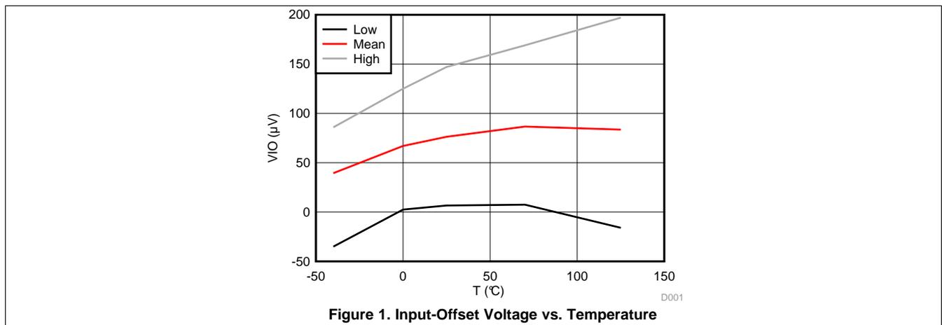
Figure 1. Input-Offset Voltage vs. Temperature
