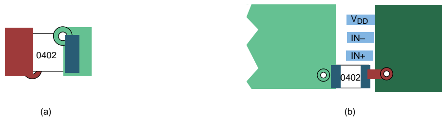
Figure 29. Typical Decoupling Capacitor Layouts
