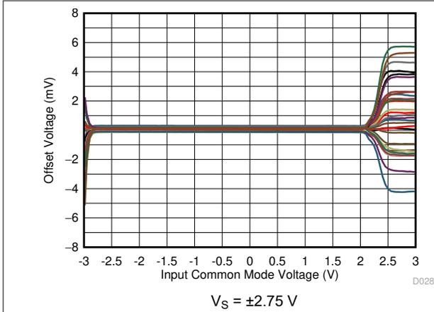
图 7-25. Input Offset vs Common Mode Voltage
