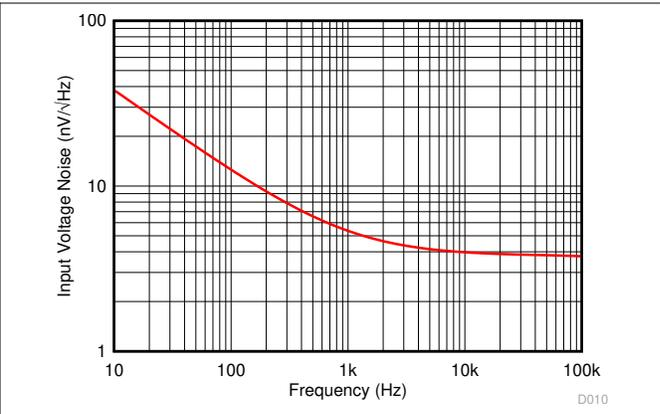
图 7-2. Input Voltage Noise Density vs Frequency
