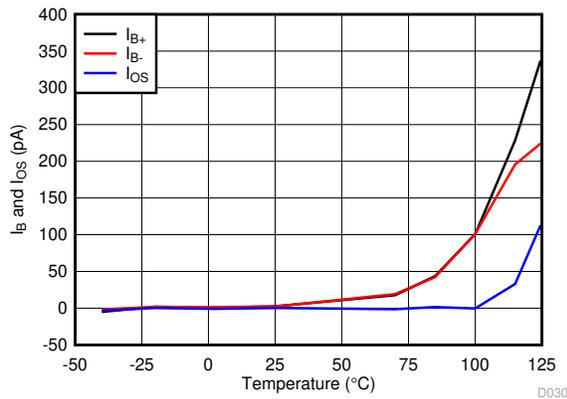
图 7-29. Input Bias and Offset Current vs Temperature
