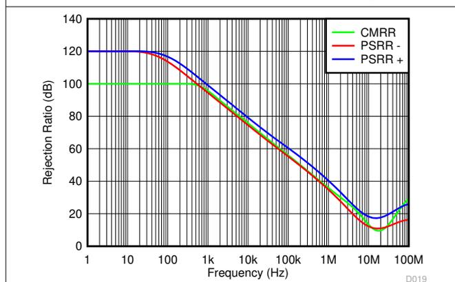
图 7-11. Rejection Ratio vs frequency
