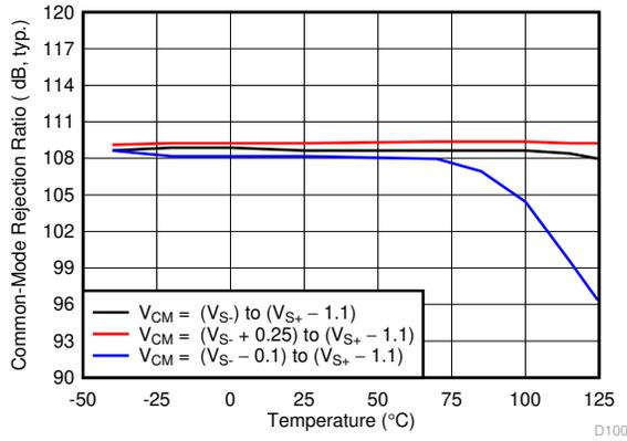
图 7-27. Common Mode Rejection Ratio vs Temperature
