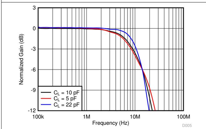
图 7-5. Small-Signal Frequency Response vs Capacitive Load
