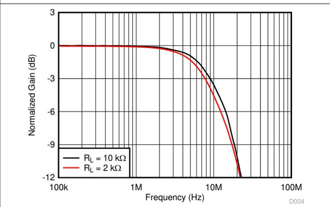
图 7-6. Small-Signal Frequency Response vs Output Load
