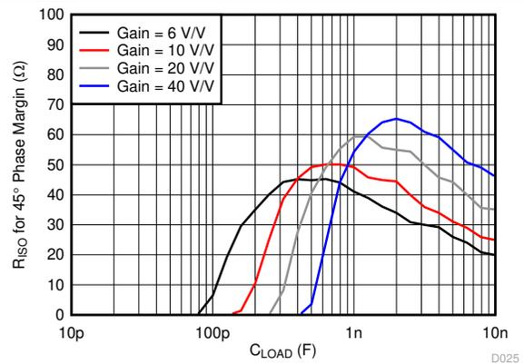
图 7-18. Recommended Isolation Resistor vs Capacitive Load
