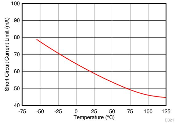
图 7-28. Short-Circuit Current vs Temperature
