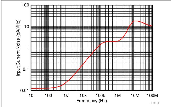
图 7-3. Input Current Noise Density vs Frequency
