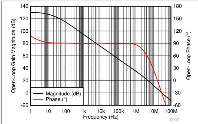
图 7-1. Open Loop Gain and Phase vs Frequency
