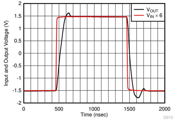
$T_{RISE} = 1\ \mu\text{sec}$ ,  $T_{FALL} = 0.7\ \mu\text{sec}$
