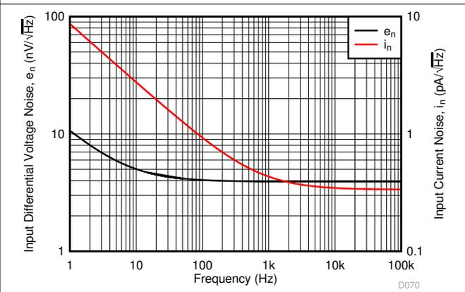
1/f corners: e<sub>n</sub> = 8 Hz, i<sub>n</sub> = 700 Hz
