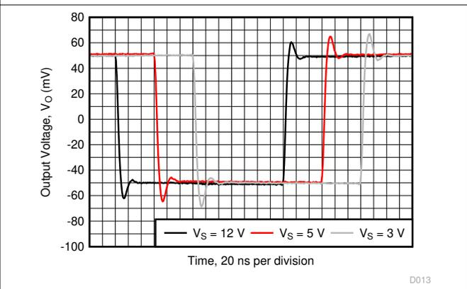
图 7-44. Small-Signal Step Response
