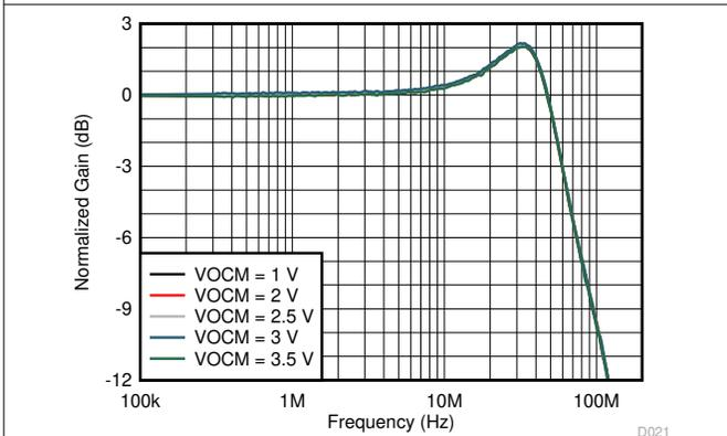
V<sub>O</sub> = 200 mV<sub>PP</sub>, see 图 8-1 with VO<sub>CM</sub> adjusted
