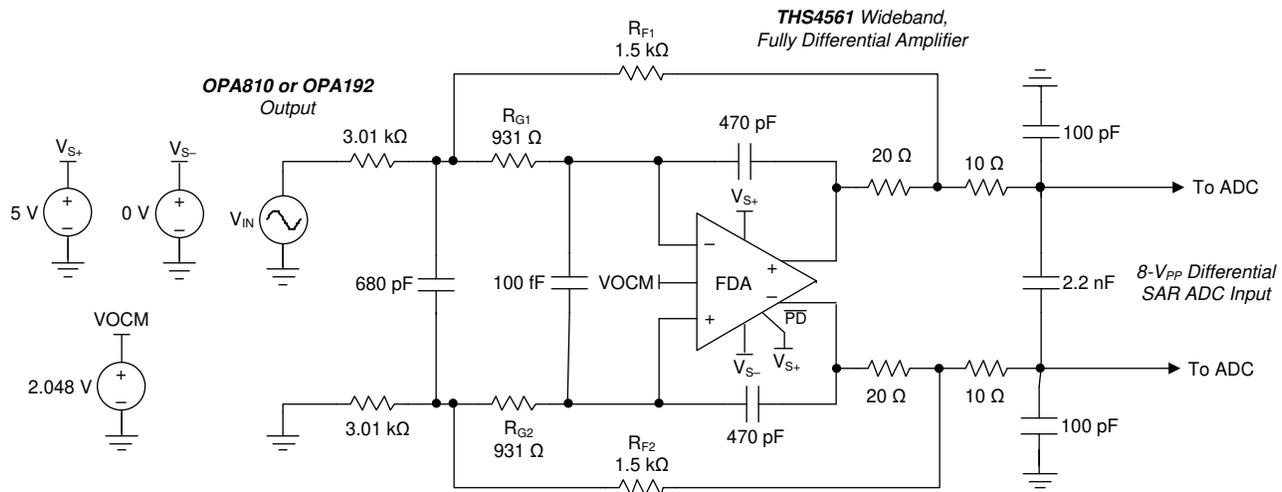
**Figure 10-7. MFB Filter Driving an ADC Application:
