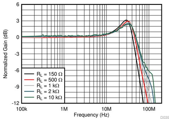
$V_O = 200\text{ mV}_{PP}$ , see 图 8-1 with  $R_L$  adjusted
