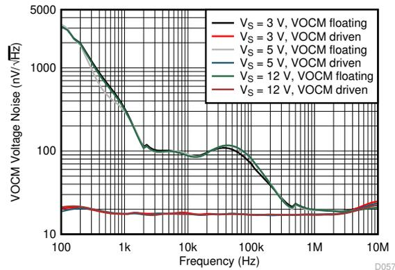
The V<sub>OCM</sub> pin is either driven to midsupply by low-impedance source or allowed to float and default to midsupply
