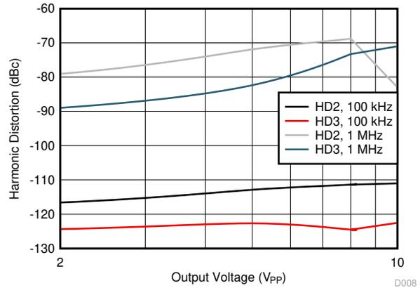
图 7-8. Harmonic Distortion vs V<sub>O</sub>
