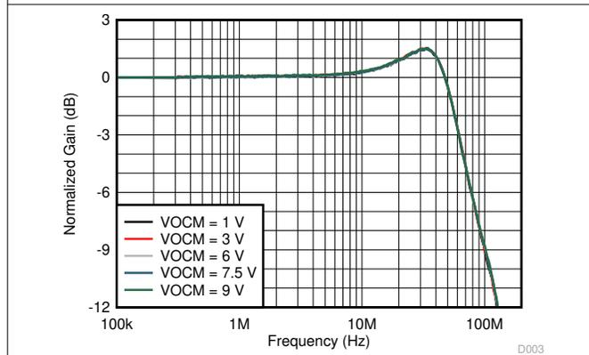
$V_O = 200\text{ mV}_{PP}$ , see [图 8-1](#) with  $V_{OCM}$  adjusted
