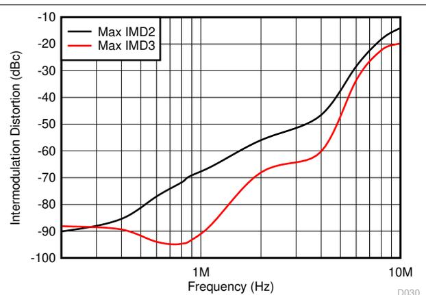
$V_O = 2\text{ V}_{PP}$  per tone,  $\pm 50\text{-kHz}$  tone spacing
