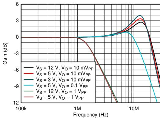
图 7-47. Common-Mode Voltage, Small-Signal and Large-Signal Response (VOCM Pin Driven)
