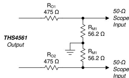
图 8-4. Output Interface for DC-Coupled Differential Outputs
