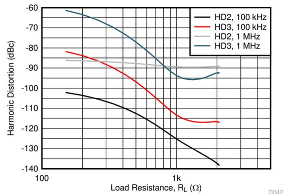
$G = 1\text{ V/V}$ ,  $V_O = 4\text{ V}_{PP}$ , with  $R_L$  adjusted
