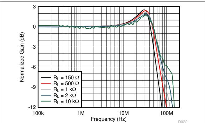
V<sub>O</sub> = 200 mV<sub>PP</sub>, see 图 8-1 with R<sub>L</sub> adjusted
