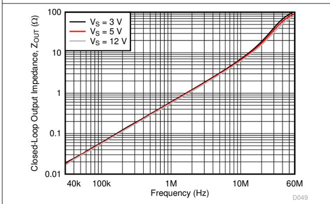
图 7-43. Closed-Loop Output Impedance vs Frequency
