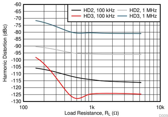
V<sub>O</sub> = 5 V<sub>PP</sub> with R<sub>L</sub> adjusted
