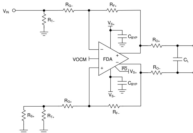
图 12-1. Representative Schematic for the Layout in
