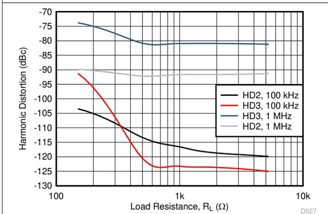
$V_O = 5\text{ V}_{PP}$  with  $R_L$  adjusted
