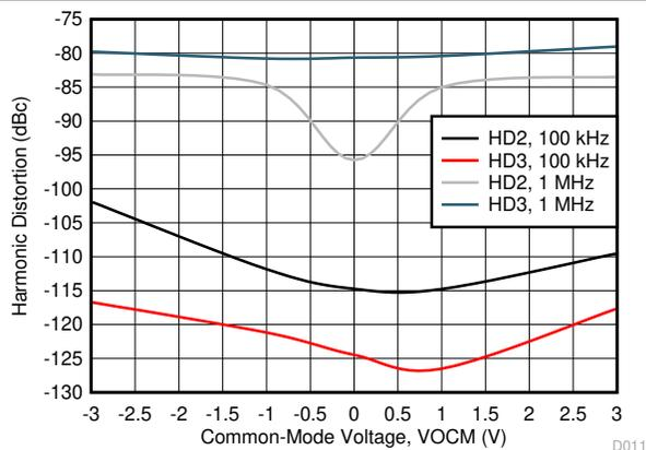
V<sub>O</sub> = 5 V<sub>PP</sub> with VO<sub>CM</sub> adjusted
