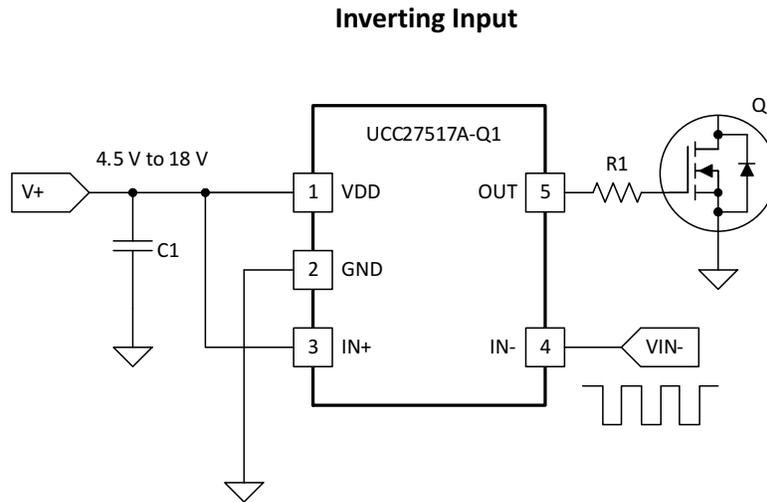
**Figure 23. Using Inverting Input (IN+ is tied to V<sub>DD</sub> enable output)**
