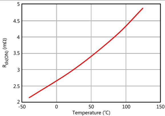
Figure 23.  $R_{DS(ON)}$  vs Temperature
