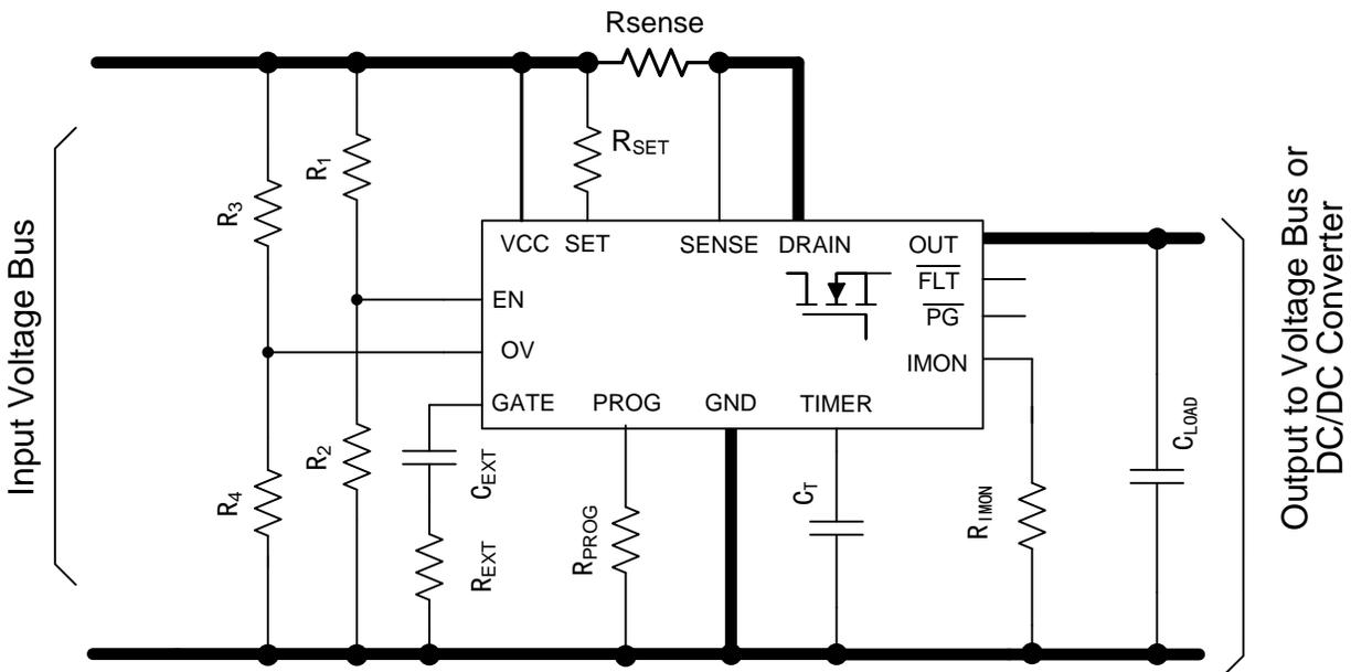
Figure 40. Gate Capacitor (dV/dt) Control Inrush Mode
