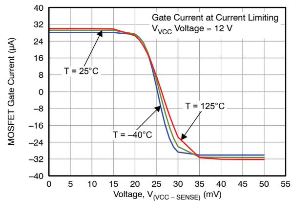
Figure 5. Internal FET Gate Current vs Voltage Across  $R_{SENSE}$  During Inrush Power Limiting
