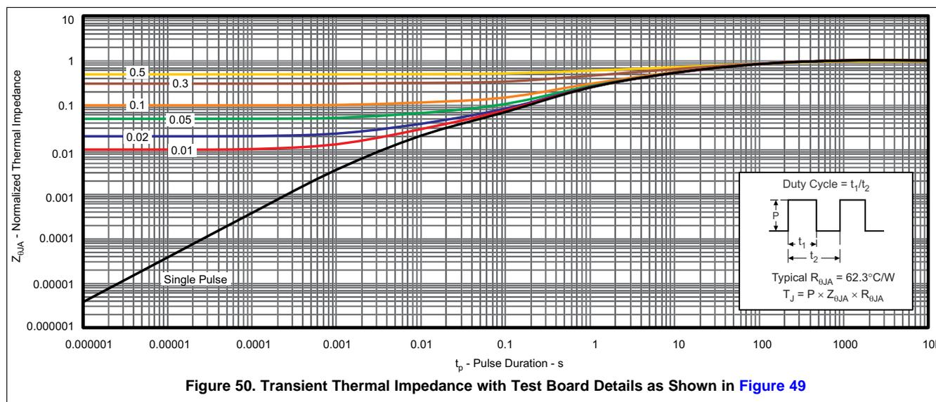
Figure 50. Transient Thermal Impedance with Test Board Details as Shown in Figure 49
