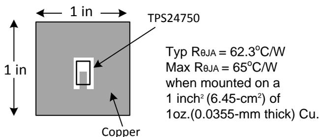
Figure 49. Board Details - Thermal Impedance Characteristic
