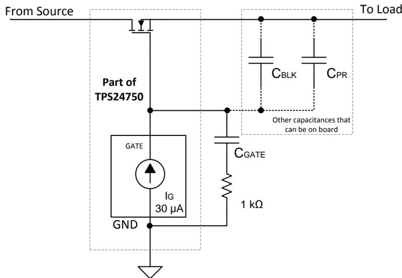
**Figure 43. Gate Capacitor (dV/dt) Control Inrush Mode.**
