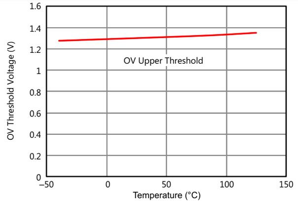
Figure 22. OV Threshold Voltage vs Temperature
