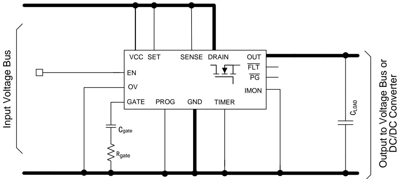
Figure 48. TPS2475x Configured as Simple 12-A Load Switch
