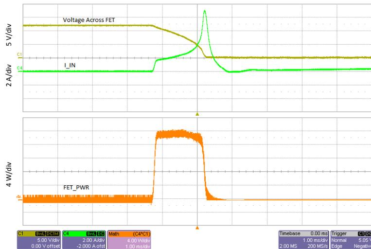
Figure 32. Computation of Power Stress During Startup
