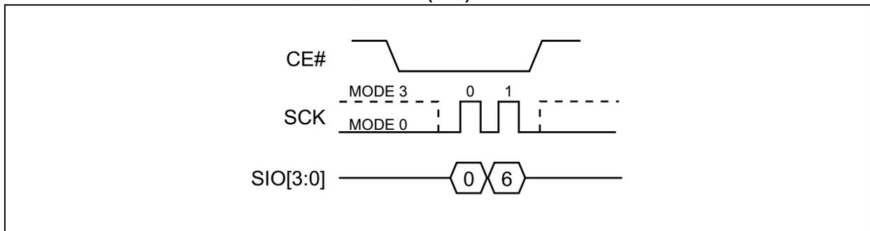
**FIGURE 5-33: WRITE ENABLE SEQUENCE (SPI)**
