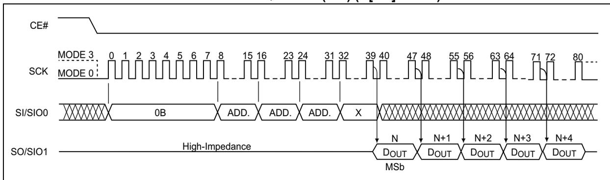
In SQI protocol, the host drives CE# low then sends one High-Speed Read command cycle, 0BH, followed by three address cycles, a Set Mode Configuration cycle and two dummy cycles. Each cycle is two nibbles (clocks) long, most significant nibble first.
