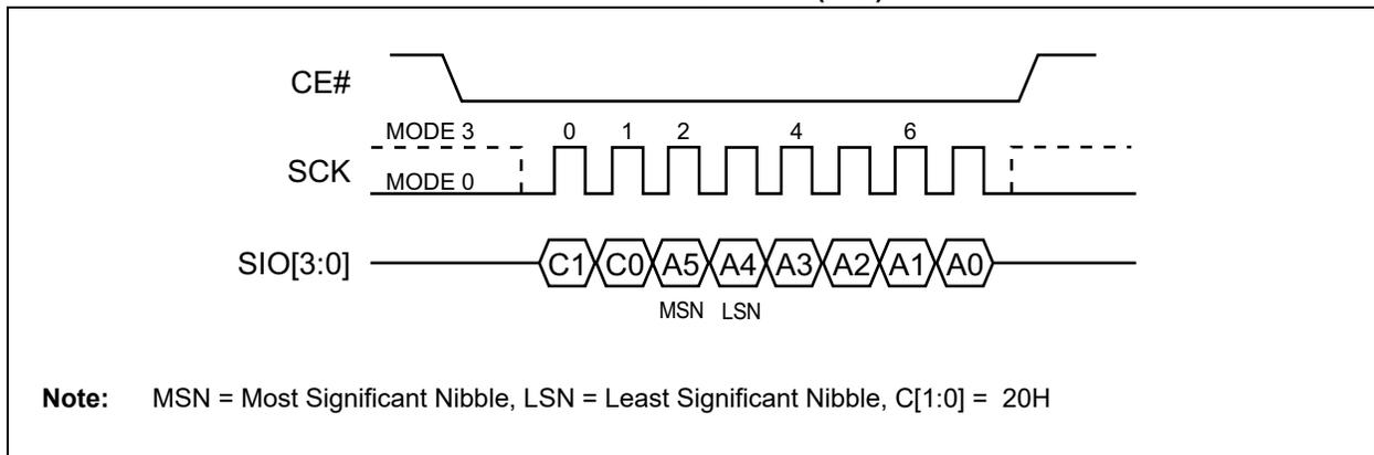
FIGURE 5-20: 4-KBYTE SECTOR ERASE SEQUENCE (SPI)
