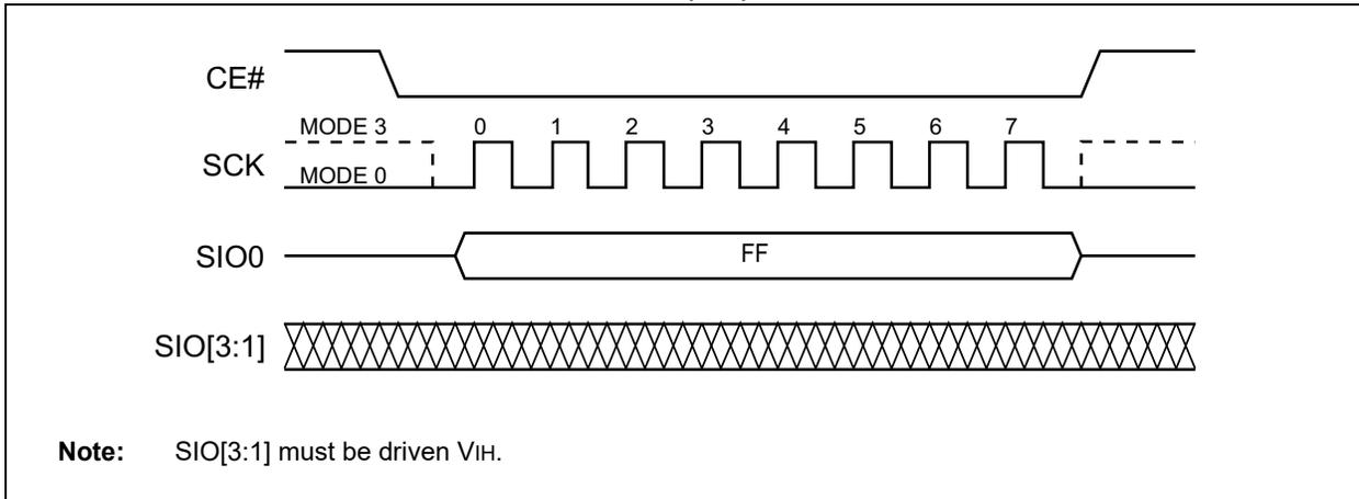
**FIGURE 5-5: RESET QUAD I/O SEQUENCE (SQI)**
