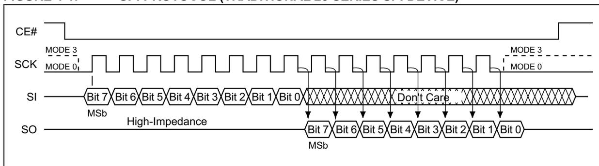
**FIGURE 4-2: SQI SERIAL QUAD I/O PROTOCOL**
