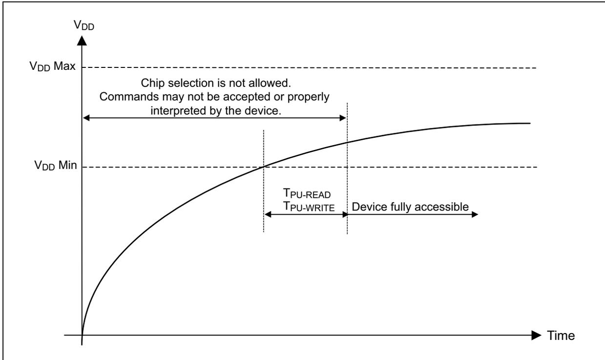
FIGURE 6-2: POWER-DOWN AND VOLTAGE DROP DIAGRAM
