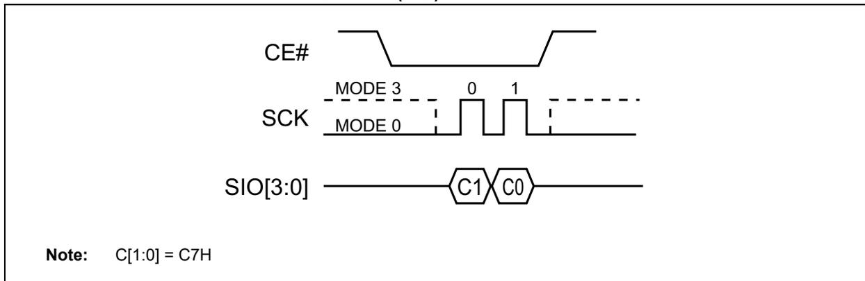
**FIGURE 5-24: CHIP ERASE SEQUENCE (SPI)**
