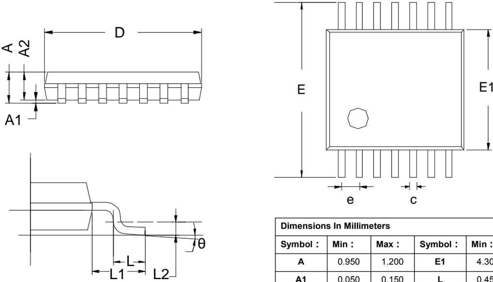
The diagram shows the TSSOP14 package with dimensions: A (lead length), A1 (lead thickness), A2 (lead thickness at base), D (width), E (height), E1 (height to top of leads), L (lead thickness), L1 (lead thickness at base), L2 (lead thickness at base), e (lead pitch), c (lead width), and θ (lead angle).
