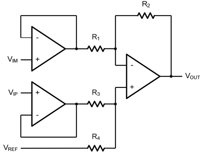
Figure 6. Instrument Amplifier
