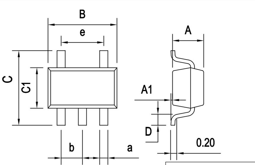
The diagram shows the SC70-5 package with dimensions labeled: B (total width), e (lead width), C (total height), C1 (body height), a (lead length), b (lead width), A (lead height), A1 (lead thickness), D (lead thickness), and Q (lead angle). A 0.20mm dimension is also indicated for the lead thickness.
