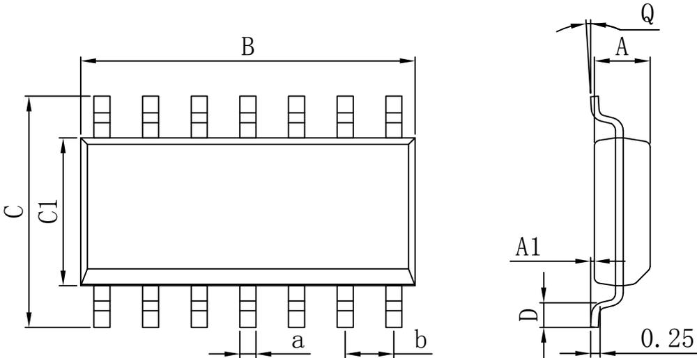
The diagram shows the SOP14 package with dimensions: B (width), C (height), C1 (height to top of leads), A (lead length), A1 (lead thickness), D (lead thickness at base), Q (lead angle), a (lead pitch), and b (lead width).
