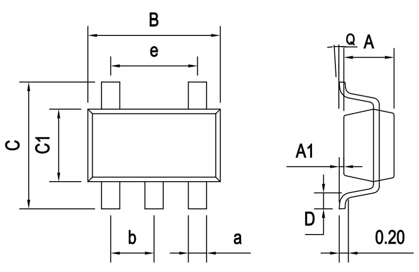
The diagram shows the SOT23-5 package with dimensions labeled: B (total width), e (lead width), C (total height), C1 (body height), a (lead length), b (lead width), A (lead height), A1 (lead thickness), D (lead thickness), and Q (lead angle). A 0.20mm dimension is also indicated for the lead thickness.
