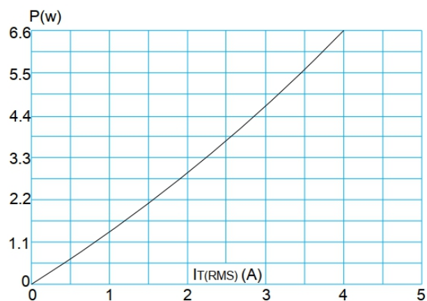
FIG.1: Maximum power dissipation versus RMS on-state current
