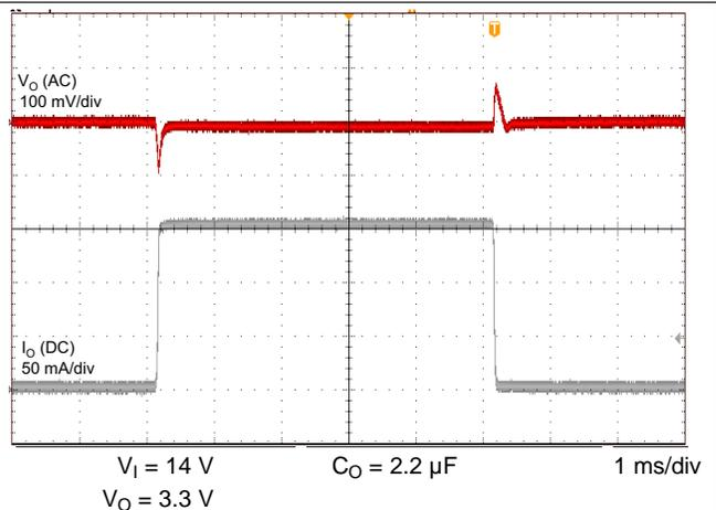
Figure 14. Load Transient (1 to 150 mA, 3.3 V)
