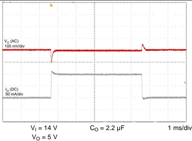
Figure 11. Load Transient (1 to 100 mA, 5 V)
