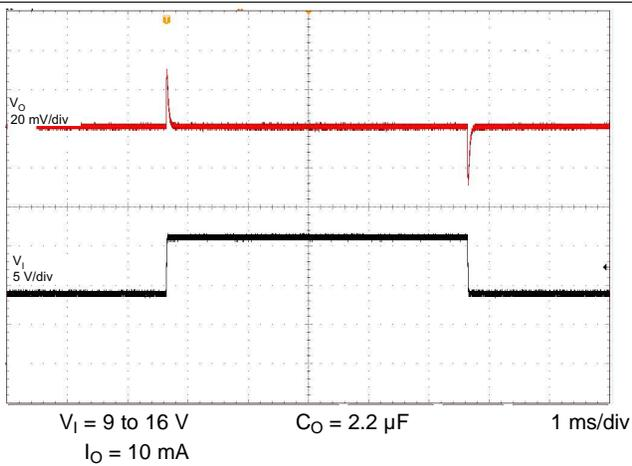
Figure 15. Line Transient ( $V_O = 5 \text{ V}$ )
