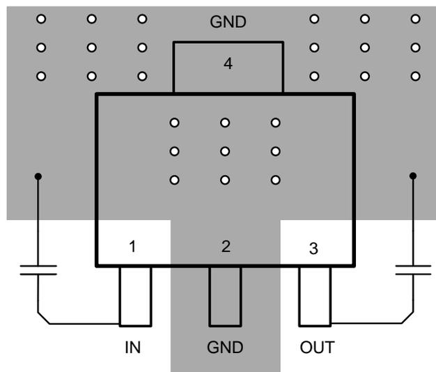
**Figure 21. Layout Example for SOT-223 Package**
