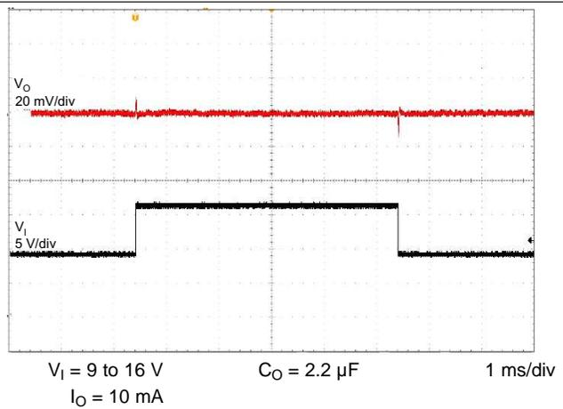
Figure 16. Line Transient ( $V_O = 3.3 \text{ V}$ )
