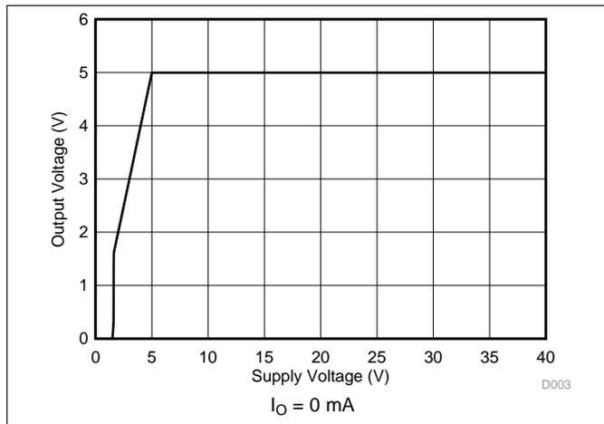
Figure 3. 5-V Output Voltage vs Supply Voltage
