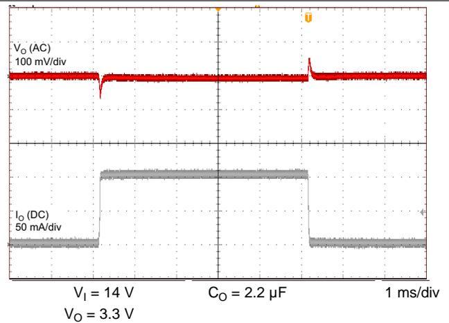
Figure 12. Load Transient (1 to 100 mA, 3.3 V)
