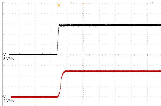
$C_O = 2.2 \mu\text{F}$ , 400  $\mu\text{s/div}$
