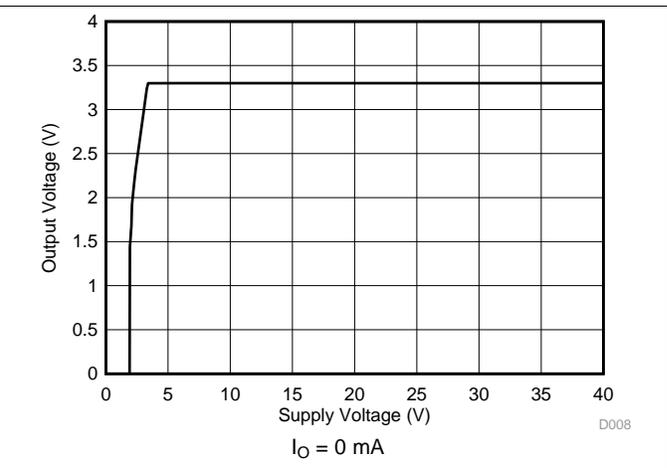
Figure 4. 3.3-V Output Voltage vs Supply Voltage
