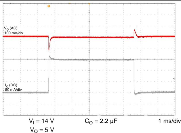
Figure 13. Load Transient (1 to 150 mA, 5 V)
