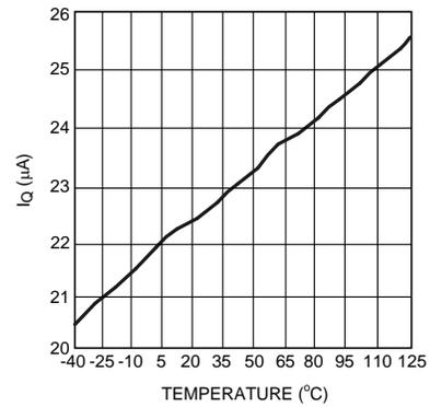
Figure 4. Quiescent Current vs Temperature (VCC = 3.3 V)
