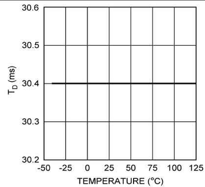
Figure 8. Time Delay (30 ms) vs Temperature
