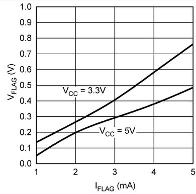
Figure 10. Flag Voltage vs Current
