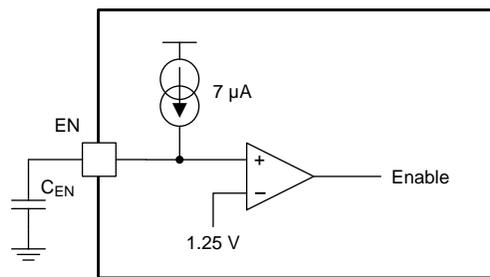
**Figure 11. Capacitor Timing**
