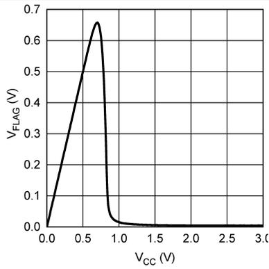
Figure 9. Flag  $V_{OL}$  vs  $V_{CC}$  ( $R_{FLAG} = 100\text{ k}\Omega$ )
