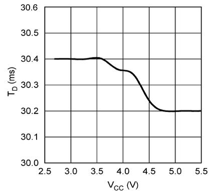
Figure 6. Time Delay (30 ms) vs VCC
