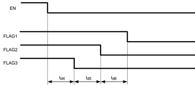
All standard options use Sequence 1 for output flags rise and fall order. Refer to section 11.1.2 for details of different sequences possible.
