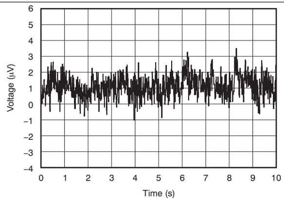
Figure 10. 0.1-Hz to 10-Hz Input Voltage Noise
