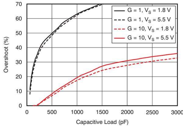
Figure 33. Small-Signal Overshoot vs Capacitive Load (100-mV<sub>PP</sub> Output Step)
