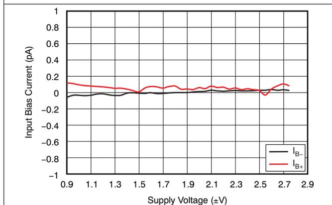
Figure 3. Input Bias Current vs Supply Voltage
