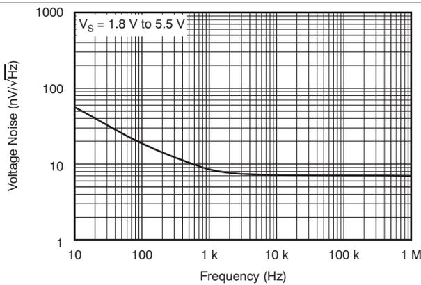
Figure 9. Input Voltage Noise Spectral Density vs Frequency
