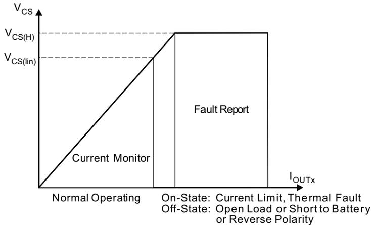
Figure 22. Current-Sense Output-Voltage Curve
