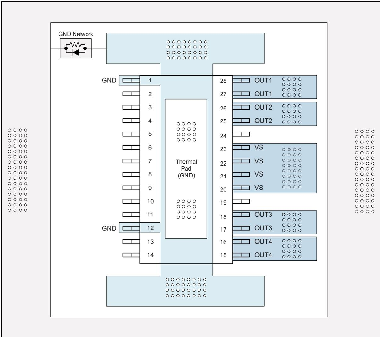
**Figure 44. Layout Example With a GND Network**
