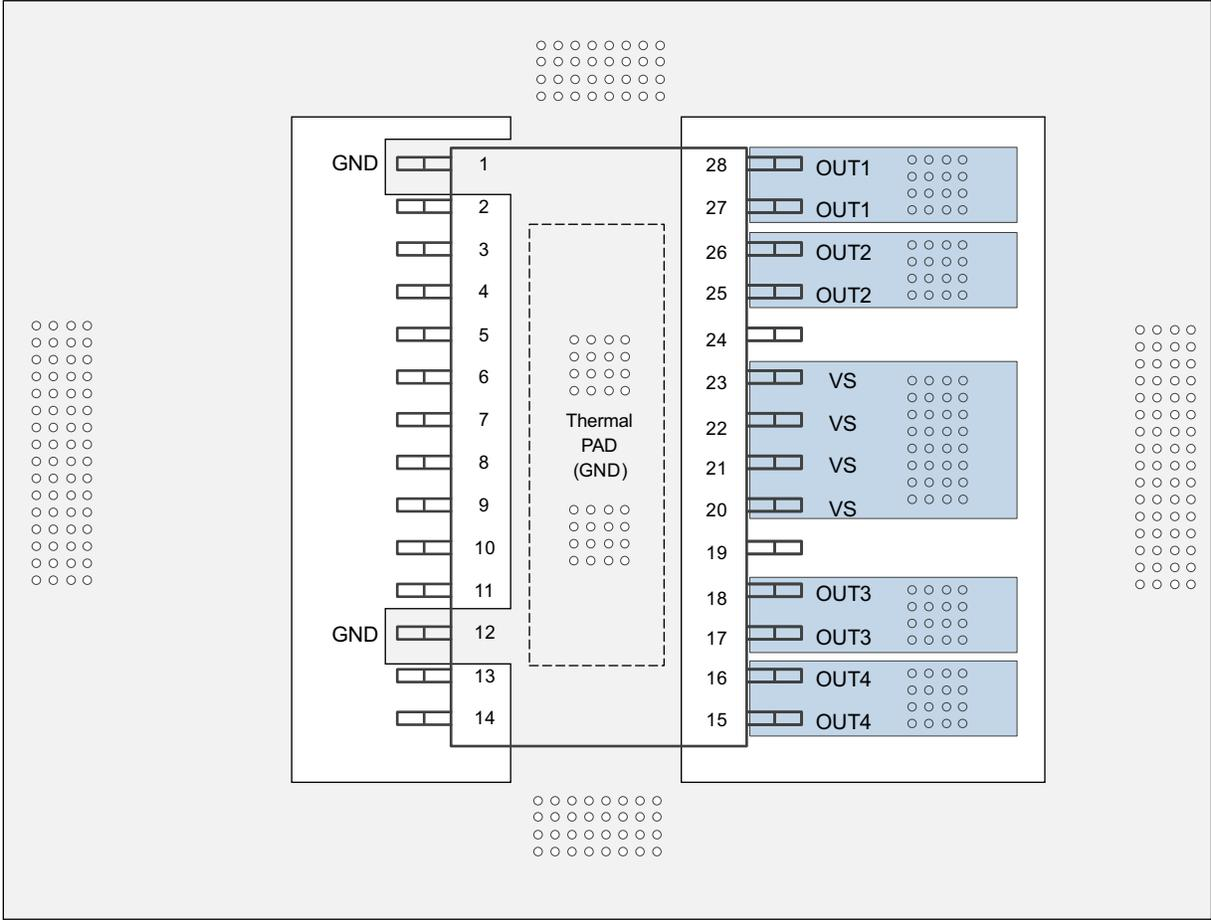
Figure 43. Layout Example Without a GND Network
