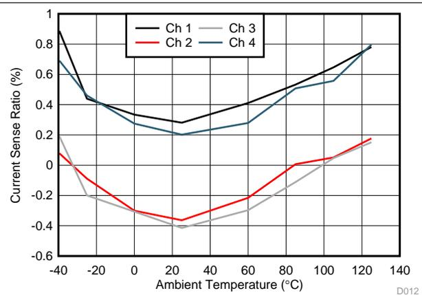
Figure 16. Current-Sense Ratio at 50 mA
