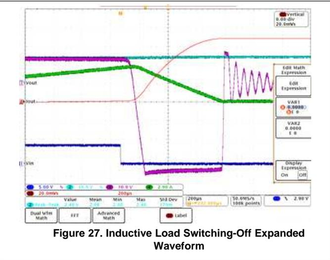
Figure 27. Inductive Load Switching-Off Expanded Waveform
