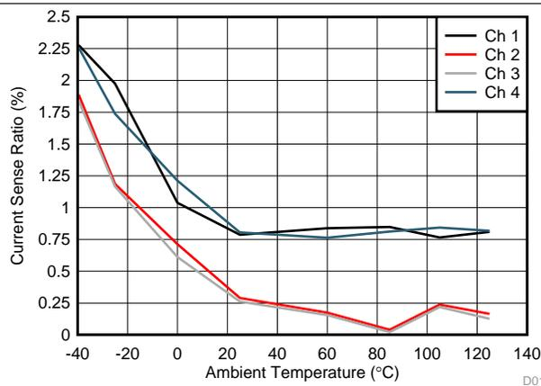
Figure 15. Current-Sense Ratio at 25 mA
